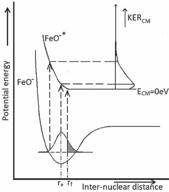
**Figure 4.** Schematic diagram describing kinetic energy release in the center-of-mass frame upon collisional excitation of the ground anion state to anion resonance.
