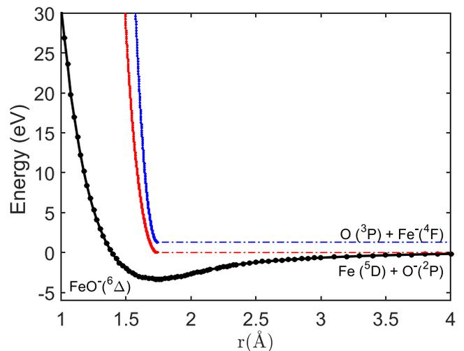
**Figure 8.** Potential energy curves for the two anion resonances accessed in the collisional excitation of  $\text{FeO}^-$ .
