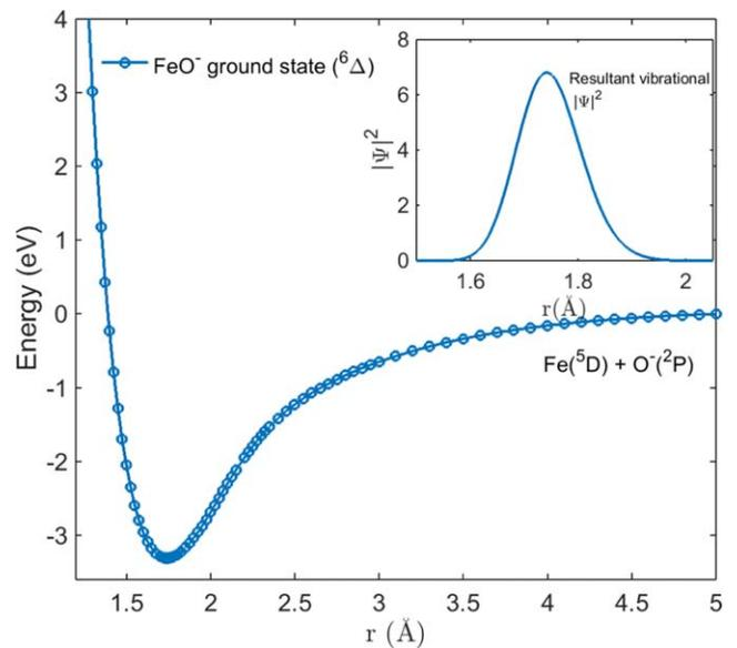
**Figure 7.** Ground electronic state of  $\text{FeO}^-$  was calculated to be  ${}^6\Delta$  using the coupled cluster method (CCSD level) using the TZV basis set. The inset shows the resultant vibrational probability density calculated using LEVEL (Le Roy 2015; see the text).
