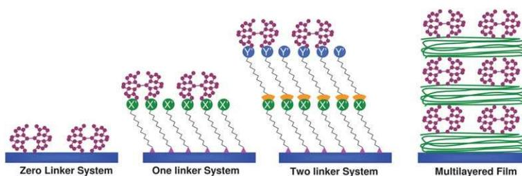
**Fig. 3** Schematic representation of dendrimer immobilization strategies on solid substrates using zero, one or two linker system and multilayered matrix fabrication.
