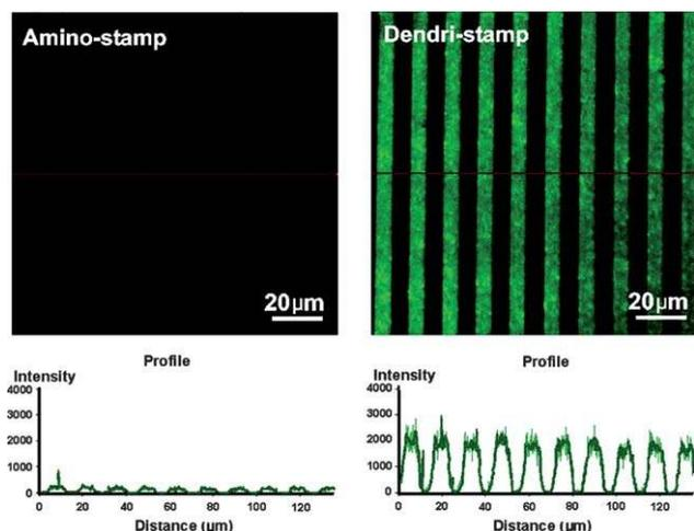
**Fig. 8** Patterns of fluorescein-labeled DNA patterns obtained by microcontact printing using an APTES-modified PDMS stamp (left) and transfer printing with a dendri-stamp (right). Reproduced with permission from Rozkiewicz *et al.*<sup>53</sup>
