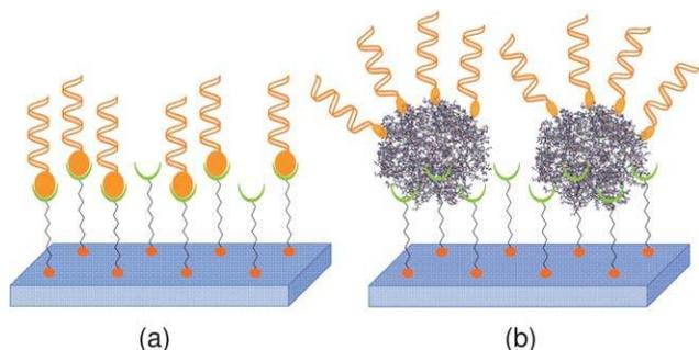
**Fig. 5** A cartoon representing the immobilization efficiency of ssDNA on (a) linear linker and (b) on dendrimer derived substrate.
