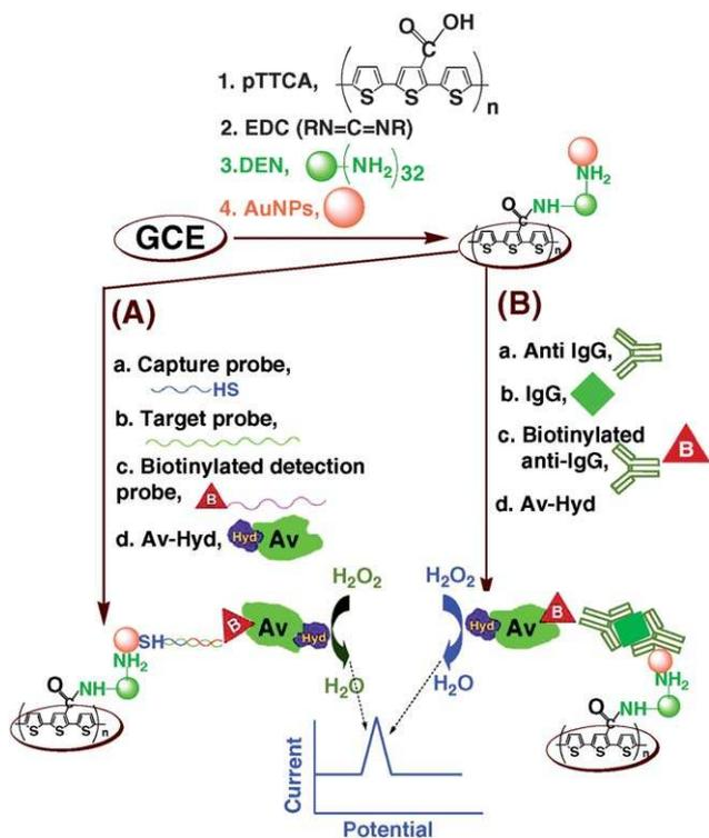
Fig. 7 Schematic presentation of the pTTCA/DEN/AuNP/biomolecules-linked avidin-hydrazine assembly for (A) DNA and (B) protein sensors, which are based on the electrocatalytic activity of hydrazine. Reproduced with permission from Shiddiky *et al.*<sup>110</sup>
