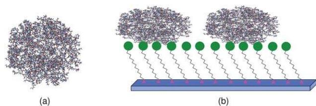
**Fig. 4** Schematic presentation of globular shaped dendrimer structure (a) in solution phase (Çağın *et al.*<sup>79</sup>) and (b) flattened or collapsed structure after immobilization on solid substrate.
