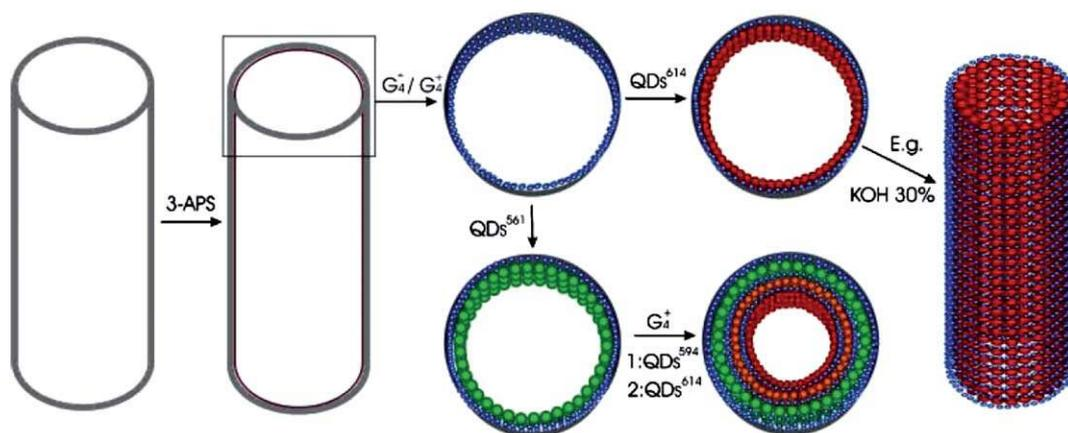
**Fig. 9** Schematic diagram of the preparation of QD/dendrimer composite NTs. Reproduced with permission from Feng *et al.*,<sup>137</sup> Copyright Wiley-VCH Verlag GmbH & Co. KGaA.
