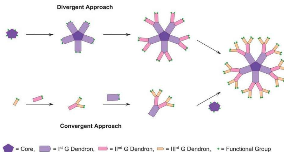
**Fig. 2** A scheme illustrating the convergent and divergent growth approach for dendrimer synthesis.
