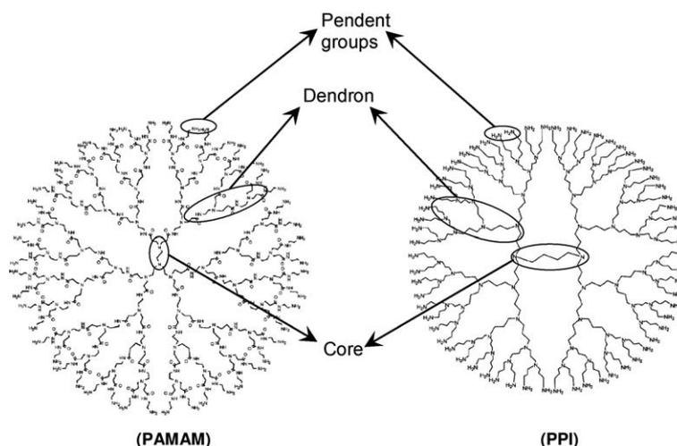
**Fig. 1** The typical structure of poly(amido amine) (PAMAM) and poly(propylene imine) (PPI) dendrimer with three distinct domains: core, dendron and pendent groups.
