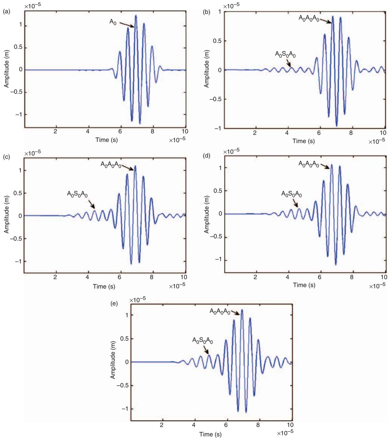
**Figure 2.** A-scans from numerical simulations on  $[0/\pm 45/90]_s$  laminate: (a) with no delamination (intact), (b) with delamination interface between plies 0, +45, (c) +45, -45, (d) -45, 90, and (e) 90, 90.
