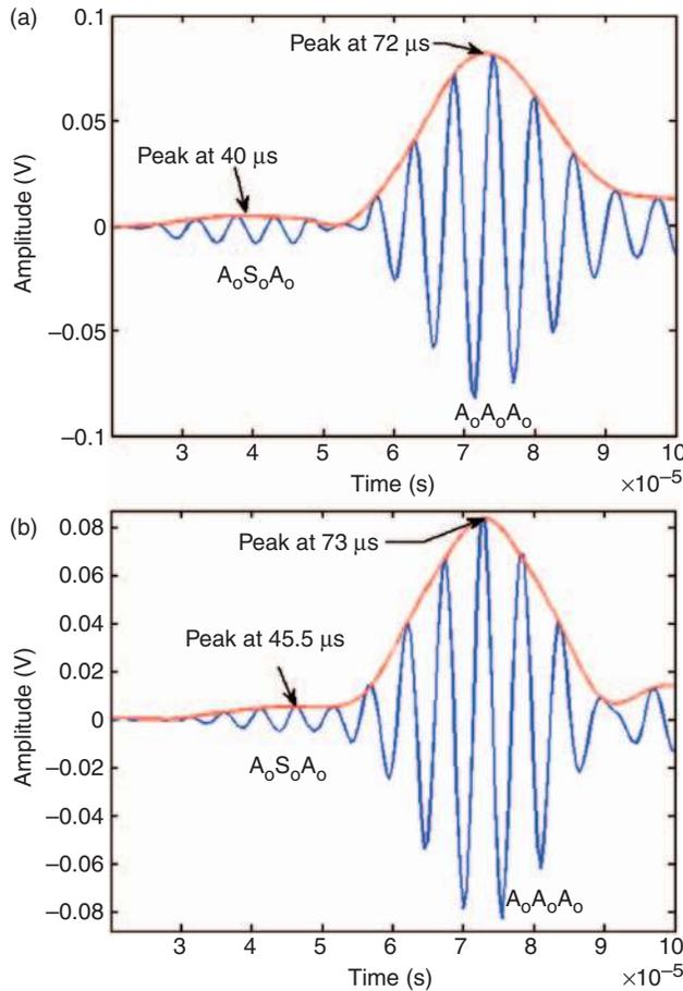
**Figure 4.** A-scans of [0/90/0] laminate: (a) 50 mm delamination and (b) 40 mm delamination.
