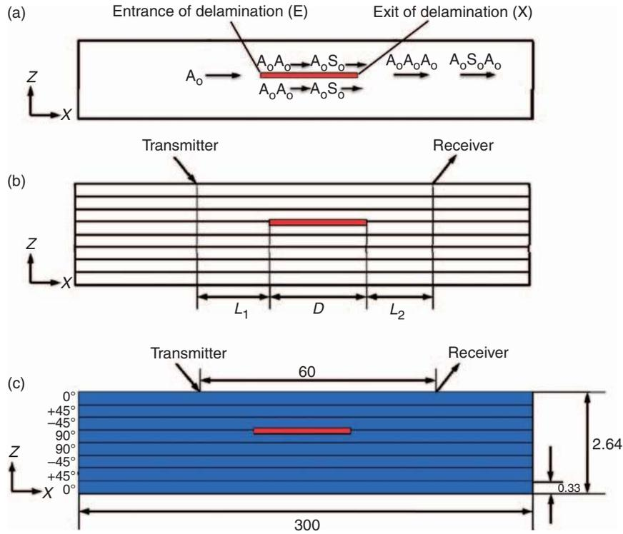
**Figure 1.** (a) Schematic of Lamb mode propagation through delamination, (b) locations of transmitter and receiver, (c) specifications of quasi-isotropic laminate.
