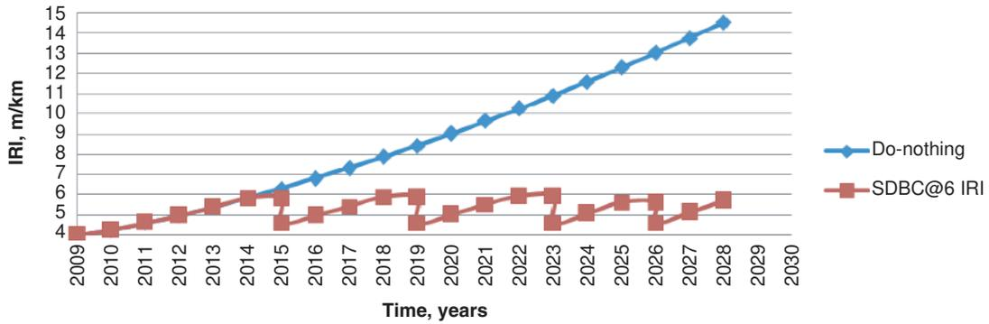
FIGURE 6 Comparison of roughness progression for doing nothing and maintenance with semidense bituminous concrete (SDBC) at 6 IRI.
