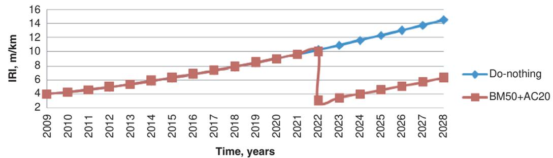
FIGURE 8 Comparison of roughness progression for doing nothing and maintenance with BM50 + asphalt concrete (AC) 20 at 10 IRI.
