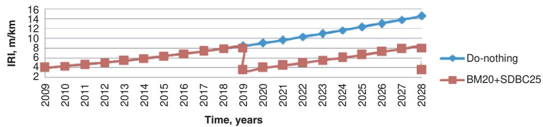
FIGURE 7 Comparison of roughness progression for doing nothing and maintenance with bituminous macadam (BM)20 + SDBC25 at 8 IRI.
