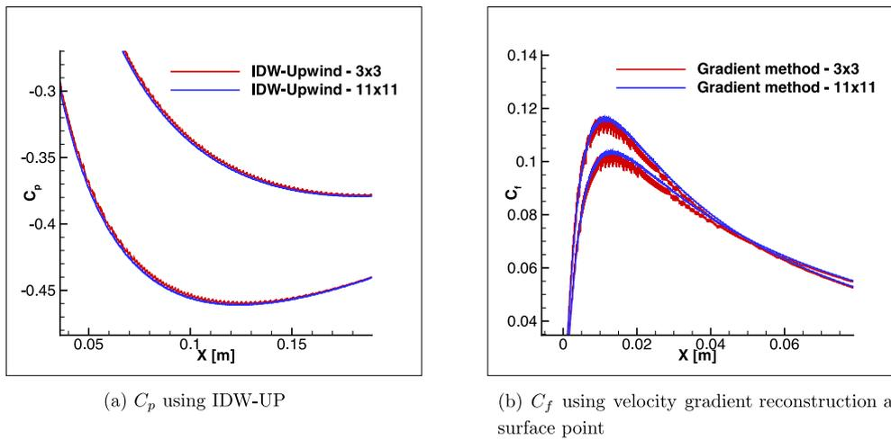
Fig. 14. Effect of stencil size on surface pressure and skin-friction coefficients for Mach 0.5 flow past NACA0012 airfoil.
