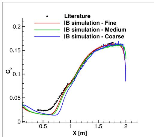
Fig. 20.  $C_p$  plot comparison across grids for Mach 3.0 flow past a  $10^\circ$  ramp
