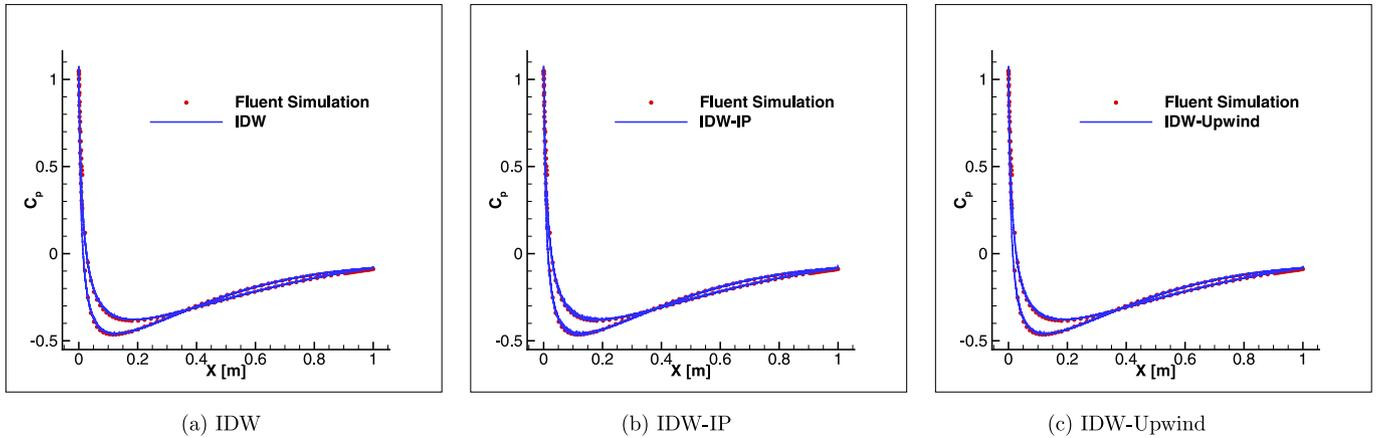
Fig. 12. Comparison of interpolation pressure reconstruction methods using  $3 \times 3$  stencil for Mach 0.5 flow past NACA0012 airfoil.
