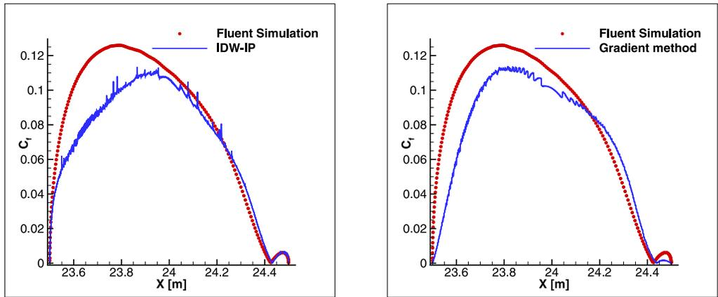
(a) Velocity reconstruction at IP using IDW-IP (b) Velocity gradient reconstruction at the surface
