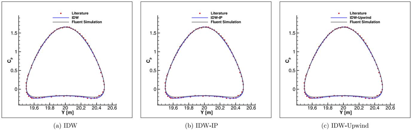
Fig. 17. Comparison of pressure interpolation methods using  $3 \times 3$  stencil for Mach 2.0 flow past circular cylinder.
