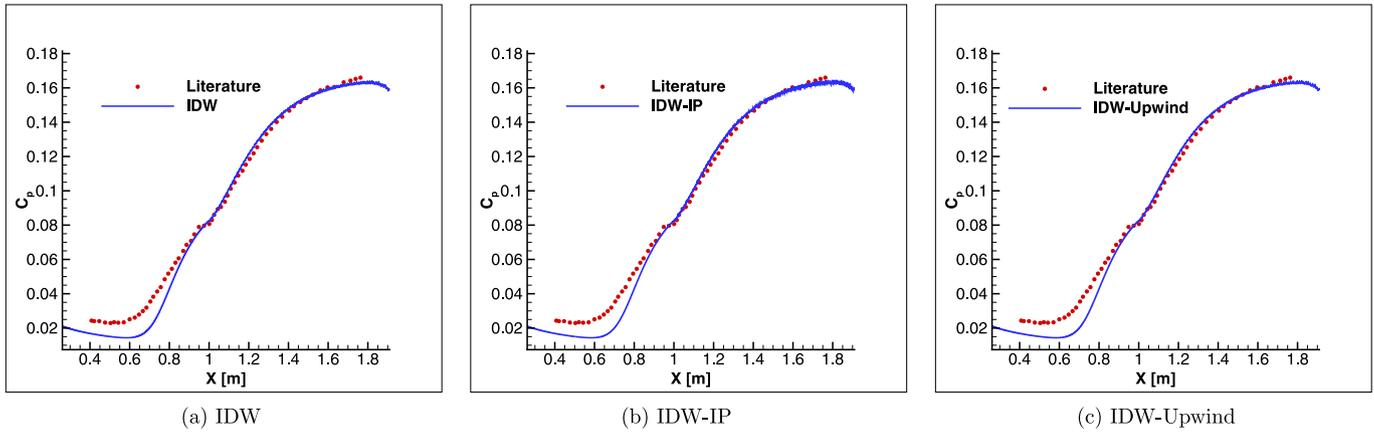
Fig. 21. Comparison of pressure interpolation methods using  $3 \times 3$  stencil for Mach 3.0 flow past a  $10^\circ$  ramp.
