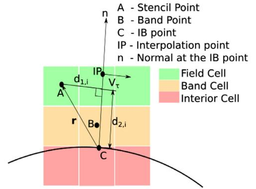
Fig. 2. Schematic of interpolation stencil for IDW-IP method.
