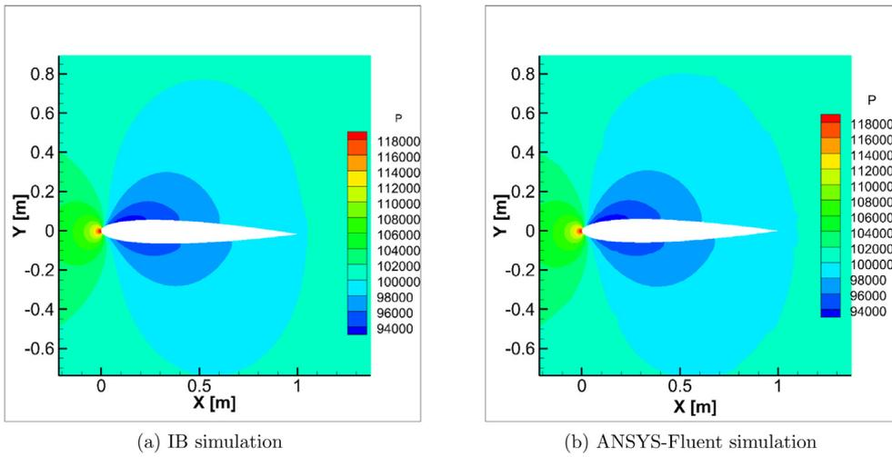
Fig. 10. Static gauge pressure contours for Mach 0.5 flow past NACA0012 airfoil.
