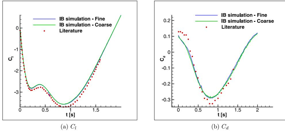
Fig. 24. Time history of force coefficients for Mach 0.2 flow past a plunging NACA0012 airfoil.
