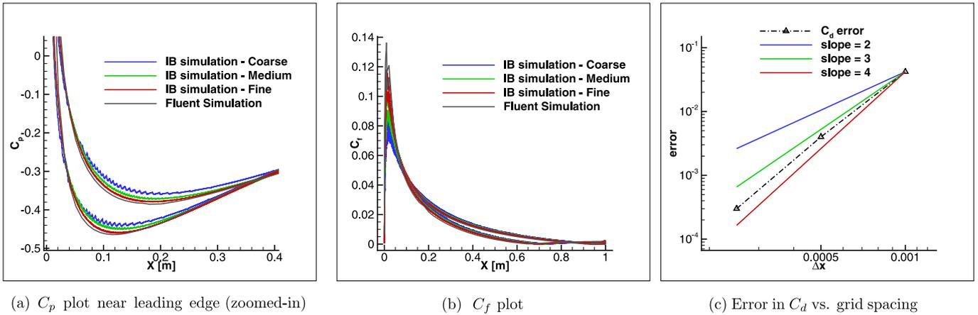
Fig. 11. Grid-convergence study for simulation of Mach 0.5 flow past NACA0012 airfoil.
