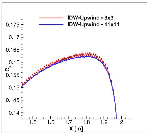
Fig. 22. Comparison of  $C_p$  using IDW-Upwind, for different stencils.
