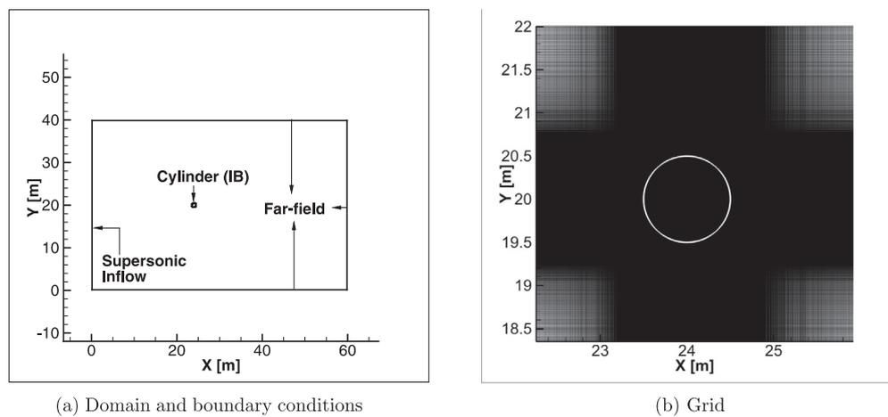
Fig. 5. Validation study: Mach 2.0 laminar flow past a circular cylinder.
