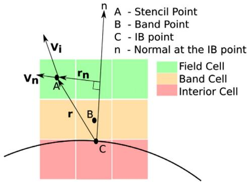
Fig. 3. Schematic of interpolation stencil for IDW-Upwind method.
