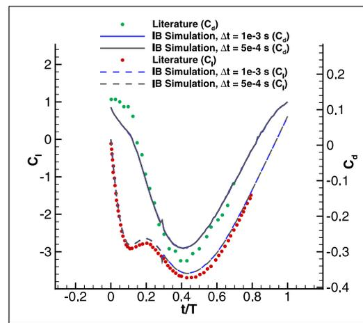
Fig. 23. Temporal convergence study for Mach 0.2 flow past plunging NACA0012 airfoil.
