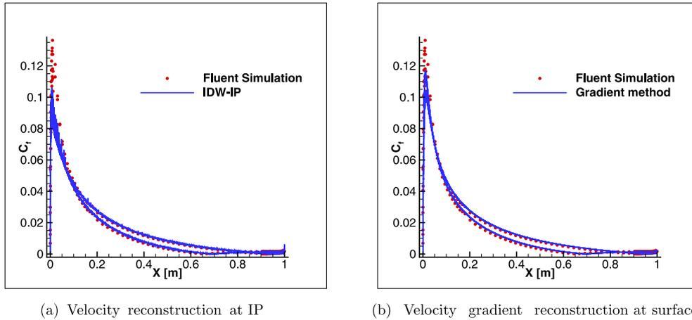
Fig. 13. Comparison shear-stress reconstruction methods using  $3 \times 3$  stencil for Mach 0.5 flow past NACA0012 airfoil.
