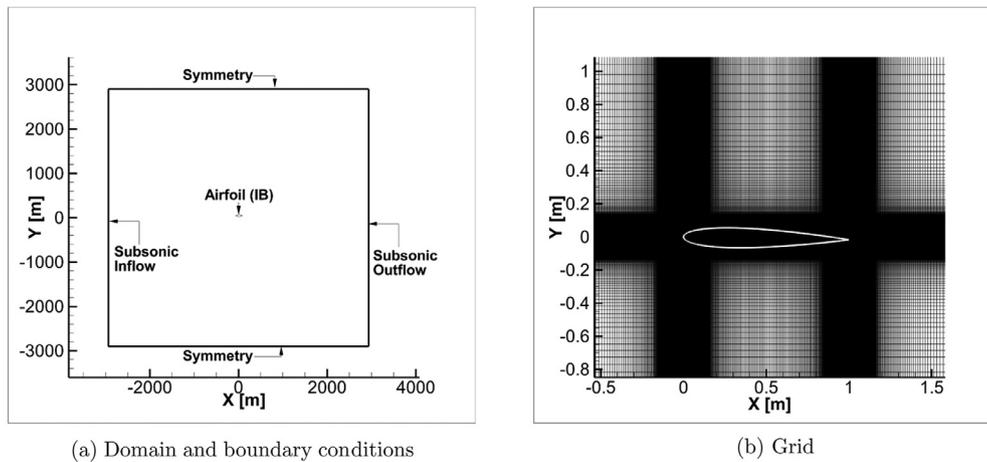
Fig. 4. Validation study: Mach 0.5 laminar flow past a NACA0012 airfoil.
