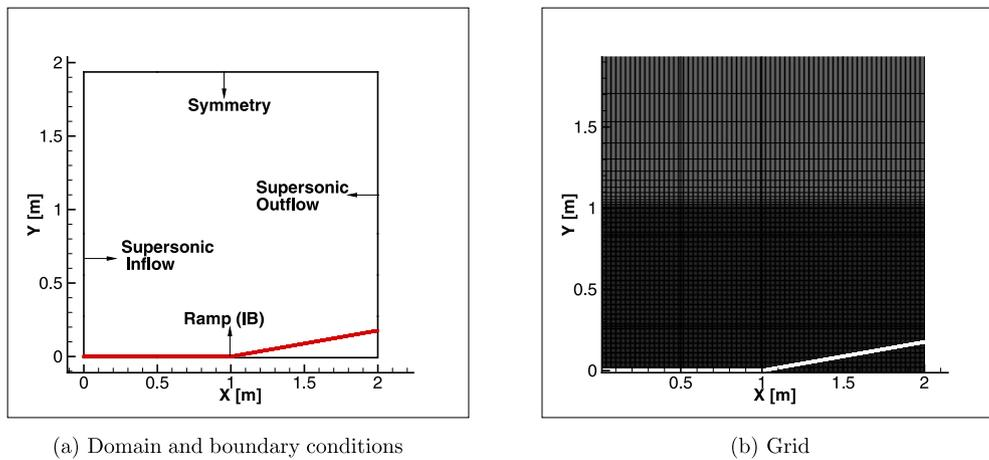
Fig. 6. Validation study: Mach 3.0 laminar flow past a  $10^\circ$  ramp.
