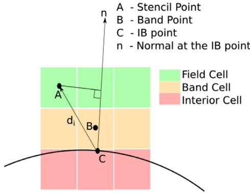
Fig. 1. Schematic of interpolation stencil for IDW method.
