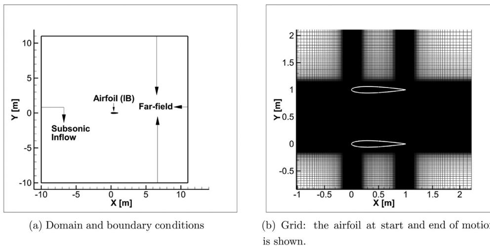
Fig. 7. Mach 0.2 laminar flow past a plunging NACA0012 airfoil.
