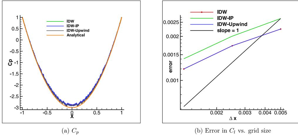
Fig. 8. Verification of surface-data interpolation for inviscid, incompressible flow past a circular cylinder.
