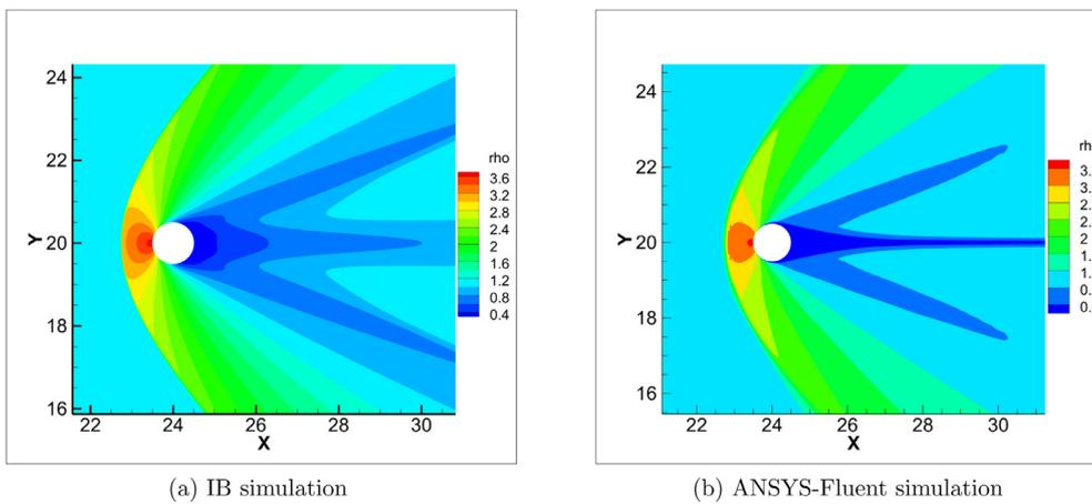
Fig. 15. Density contours of Mach 2.0 flow past circular cylinder.
