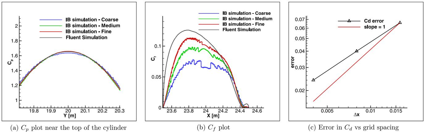
Fig. 16. Grid-convergence study for Mach 2 supersonic flow past a circular cylinder.
