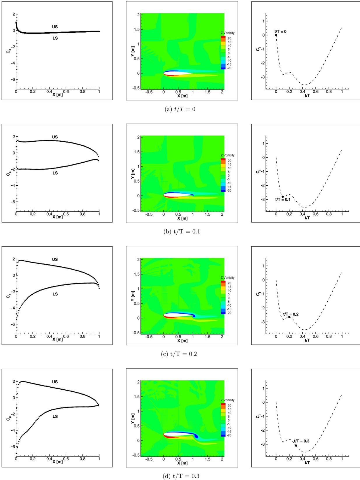
**Fig. 25.**  $C_p$  distribution (left), vorticity contours (middle), and  $C_l$  (right) at different times for Mach 0.2 flow past a NACA0012 plunging airfoil:  $t/T = 0.0$ – $1.0$ ; US – Upper Surface, LS – Lower Surface.
