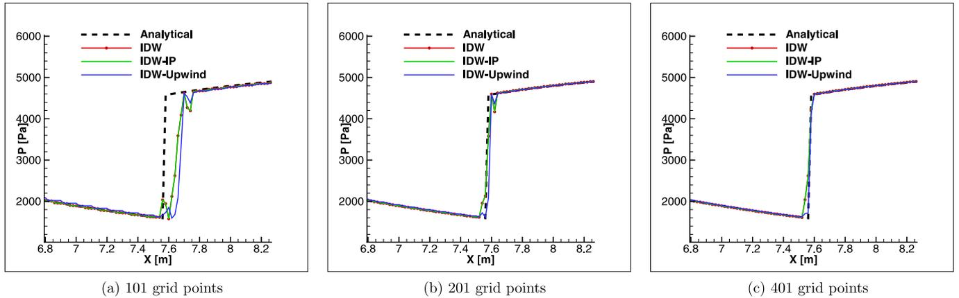
Fig. 9. Interpolated pressure distribution in a CD nozzle with pressure ratio 0.75.
