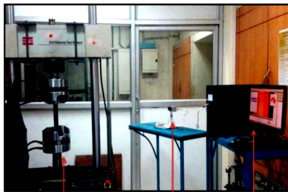
Fig. 4 – Infrared imaging and MTS 810 servo-hydraulic test system used for the experiments.
