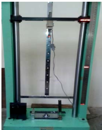
Fig. 3 – Drop Impact tester used for impacting specimens.
