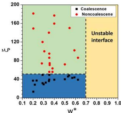
**FIG. 6.** The magnetophoretic coalescence and noncoalescence regimes are characterized based on the ratio of the width of the ferrofluid stream to that of the channel width ( $w^*$ ) and the ratio of total migration time scale to the advection time scale  $\xi$ . Magnetocoalescence of droplets is observed for  $w^* < 0.7$  (stable interface) and  $\xi \leq 50$ , and the boundaries demarcating the various regimes are identified by analyzing the experimental data.
