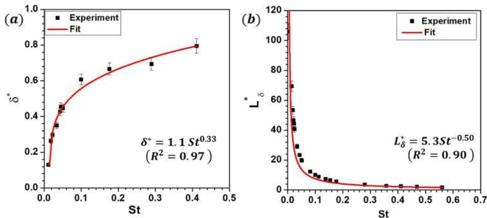
**FIG. 3.** (a) The variation of the magnitude of dimensionless equilibrium cross-stream migration distance  $\delta^* = (\delta/w)$  with the Stouhal number  $St = (\tau_a/\tau_m)$ . (b) The variation of the dimensionless length required for attaining the equilibrium location  $L_\delta^* = (L_\delta/w)$  with the Stouhal number  $St$ .
