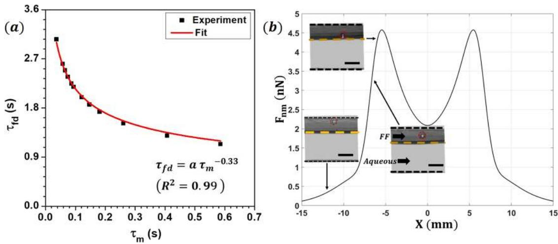
**FIG. 5.** (a) Interdependency of time scales  $\tau_m$  and  $\tau_{fd}$ : if  $\tau_m$  increases, then  $\tau_{fd}$  decreases and vice versa. (b) Variation in the magnetic force along the flow direction and images of the cross-stream migration and coalescence of droplets are shown in the inset.
