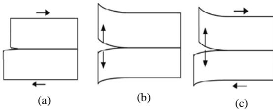
Fig. 1 Modes of bond failures: (a) Shear separation (Mode A) (b) Tensile separation (Mode B) (c) Mixed shear and tensile separation (Mode C)
