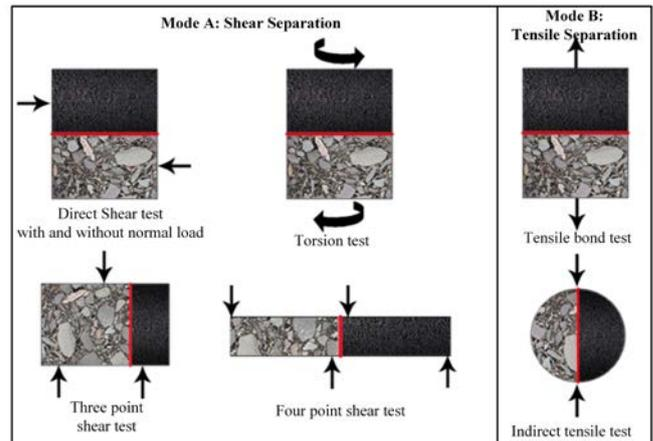
Fig 3. Interface bond test methods
