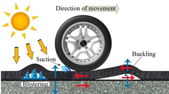
Fig 2. The field mechanism of bond failures
