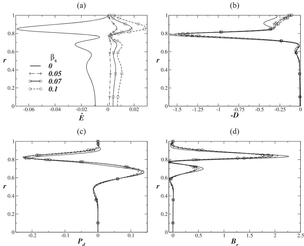
FIG. 4. Radial variations of (a) the rate of change of kinetic energy,  $\dot{E}$ , (b) the negative of the dissipation rate ( $-\mathcal{D}$ ), (c) the production rate,  $P_d$ , and (d)  $\mathcal{B}_r$  of the most dangerous modes at  $A_1$ ,  $B_1$ ,  $C_1$ , and  $D_1$  in Fig. 3(a) for different values of  $\beta_s$ , respectively. The rest of the parameter values are the same as in Fig. 3(a).
