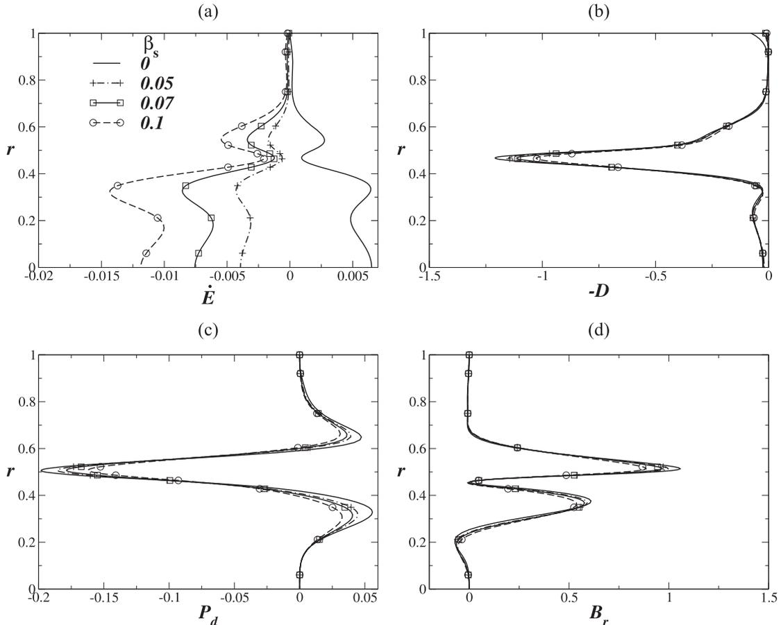
FIG. 5. Radial variations of (a) the rate of change of kinetic energy,  $\dot{E}$ , (b) the negative of the dissipation rate ( $-D$ ), (c) the production rate,  $P_d$ , and (d)  $B_r$  of the most dangerous modes at  $A_2$ ,  $B_2$ ,  $C_2$ , and  $D_2$  in Fig. 3(b) for different values of  $\beta_s$ , respectively. The rest of the parameter values are the same as in Fig. 3(b).
