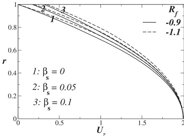
FIG. 12. Basic velocity profiles in a DD flow configuration when  $R_1 = 0.7$  and  $q = 0.1$  with less viscous fluid ( $R_f = -1.1$ ,  $R_s = 1$ ; dashed line) and more viscous fluid ( $R_f = -0.9$ ,  $R_s = 1$ ; solid line) in the annular region.
