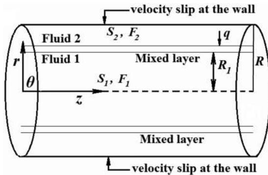
FIG. 2. Schematic diagram of the problem considered. The core ( $0 \leq r \leq R_1$ ) and the annular ( $R_1 + q \leq r < R$ ) regions of the slippery pipe contain fluids “1” and “2,” respectively. A mixed layer of thickness  $q$  occupies the region  $R_1 \leq r \leq R_1 + q$ . There is velocity slip at the walls of the pipe ( $r = R$ ).
