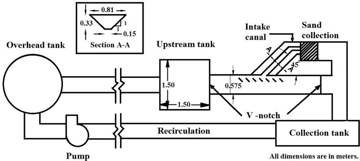
FIGURE 1. Schematic diagram of the experimental setup
