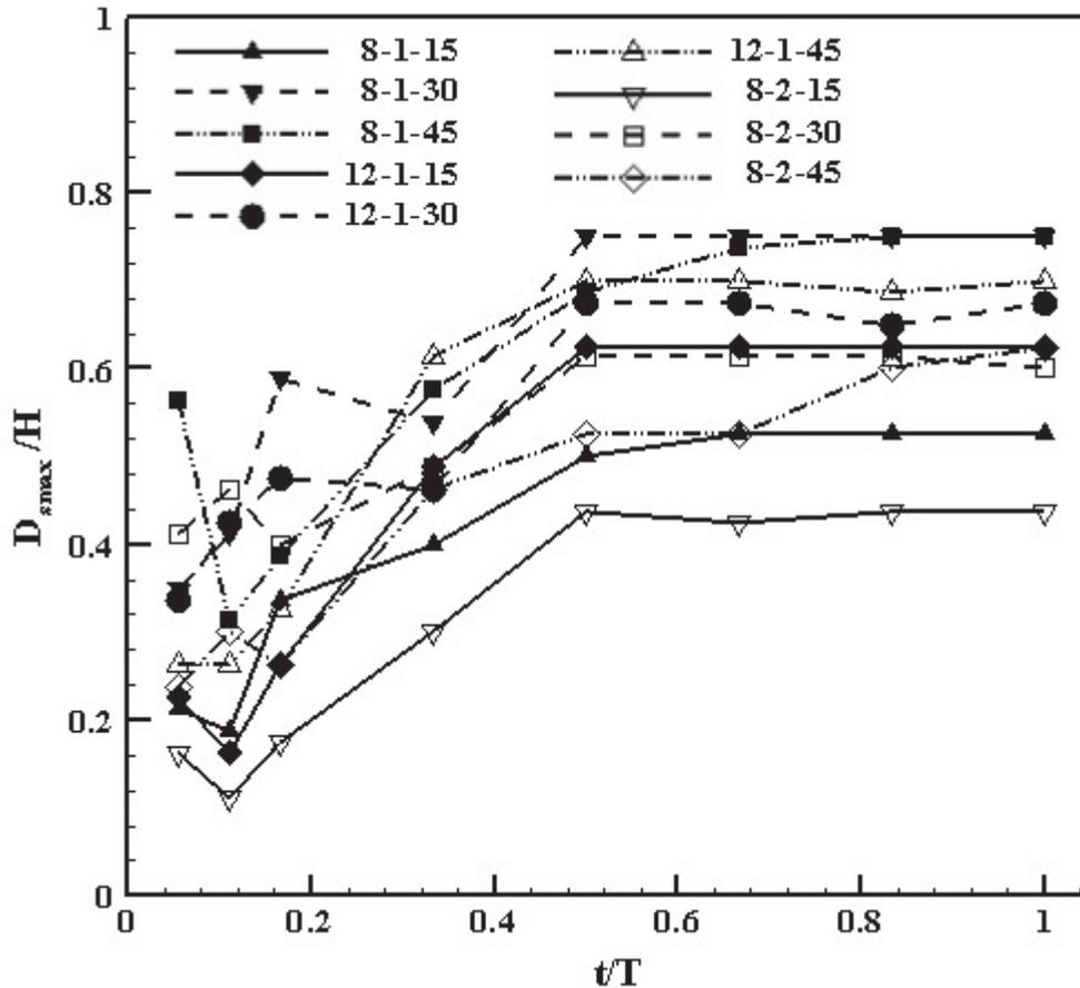
FIGURE 2. Variation of local scour ratio with time for different vane arrangements
