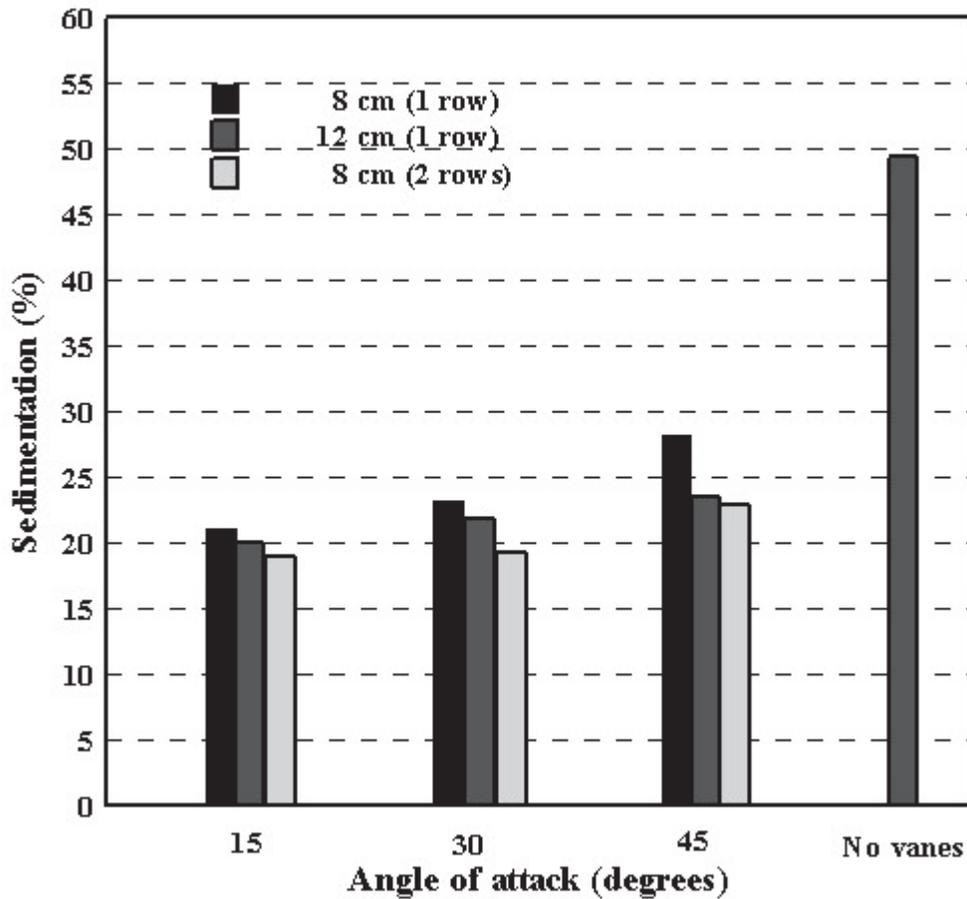
FIGURE 3. The variation of sedimentation (%) for different arrangement
