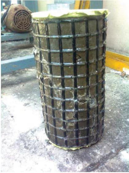
Figure 4 Compression failure of specimen confined with FABpoly
