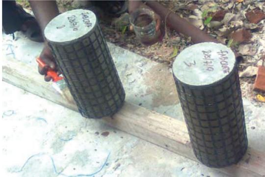
Figure: 2(a) Cylindrical concrete specimen confined with FABpoly
