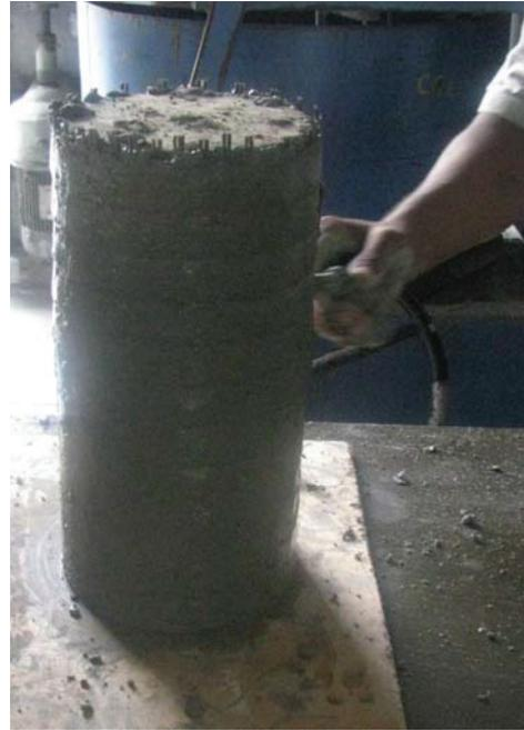
Figure: 2(b) Cylindrical concrete specimen confined with FABcrete
