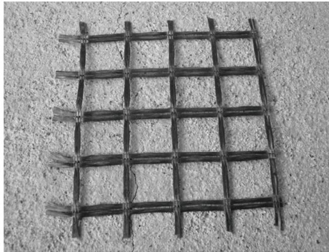
Figure 1: Architecture of glass fabric
