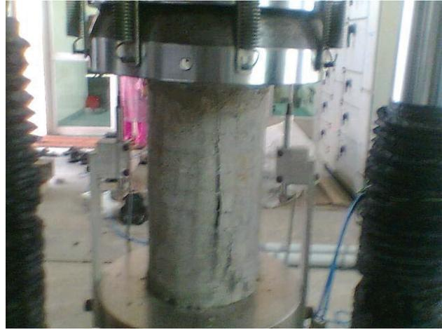
Figure 5: Compression failure of specimen confined with FABcrete
