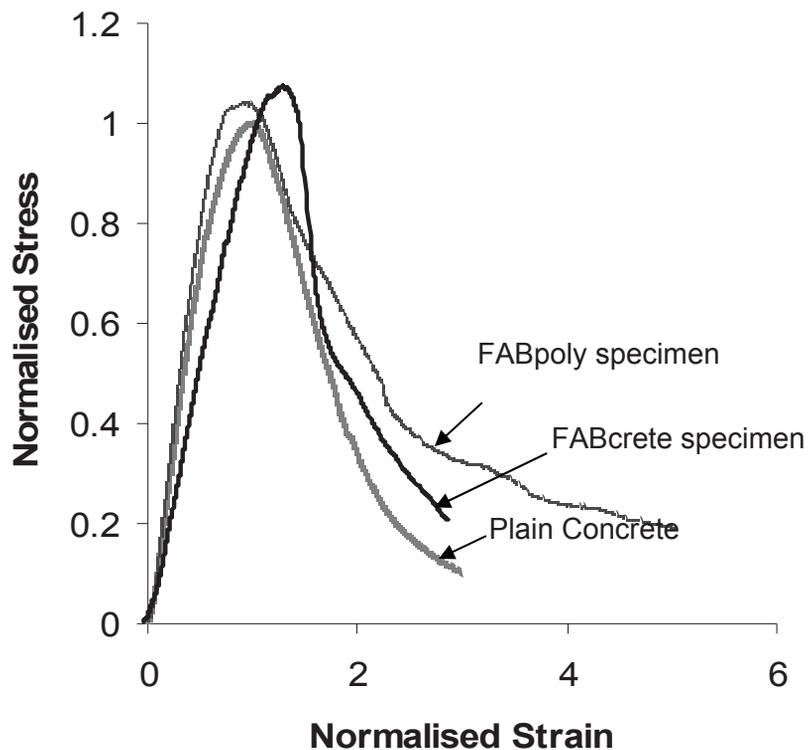
Figure: 3 Stress-strain behaviour of confined and unconfined specimens
