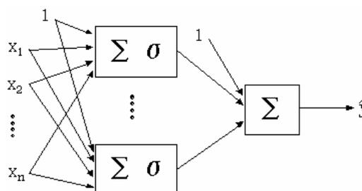
Fig.1 Architectural representation of feed forward neural network
