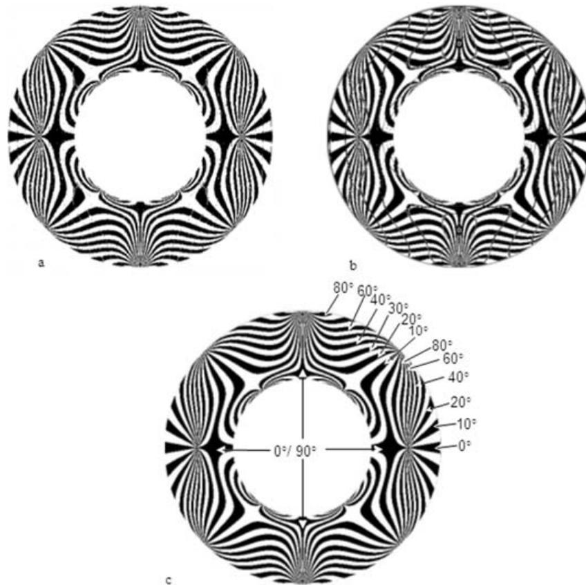
**Fig. 2** Isoclinic plots in steps of  $10^\circ$  obtained from theoretically simulated phase-shifted/polarization-stepped images of a ring under diametral compression. (a) Representative plot for circular and mixed polariscope arrangements, (b) representative plot for plane polariscope arrangements, and (c) analytical solution [29]
