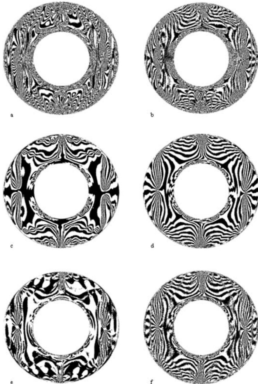
**Fig. 3** Isoclinic plots in steps of  $10^\circ$  obtained from the experimentally recorded phase-shifted/polarization-stepped images of a ring under diametral compression by: (a) Patterson and Wang, (b) Ajovalasit *et al.*, (c) Mangal and Ramesh, (d) Brown and Sullivan, (e) Chen and Lin (without adjustment), (f) Chen and Lin (with adjustment), (g) Sarma *et al.*, (h) Dupré *et al.*, (i) Kihara, (j) Petrucci, and (k) Lei Zhenkun *et al.*
