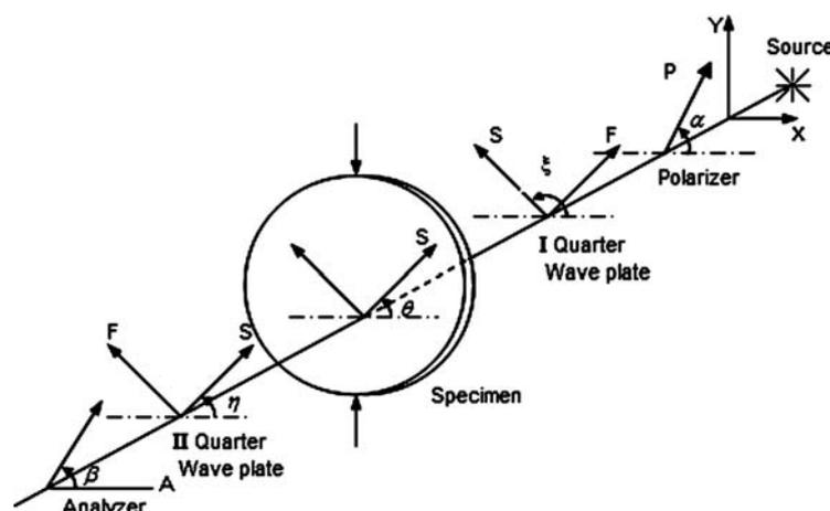
Fig. 1 Generic arrangement of a circular polariscope to employ phase-shifting methodology
