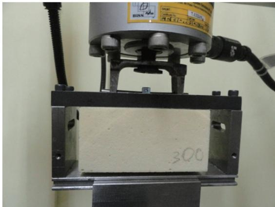
**Fig. 3.** Setup for pull-out strength study.
