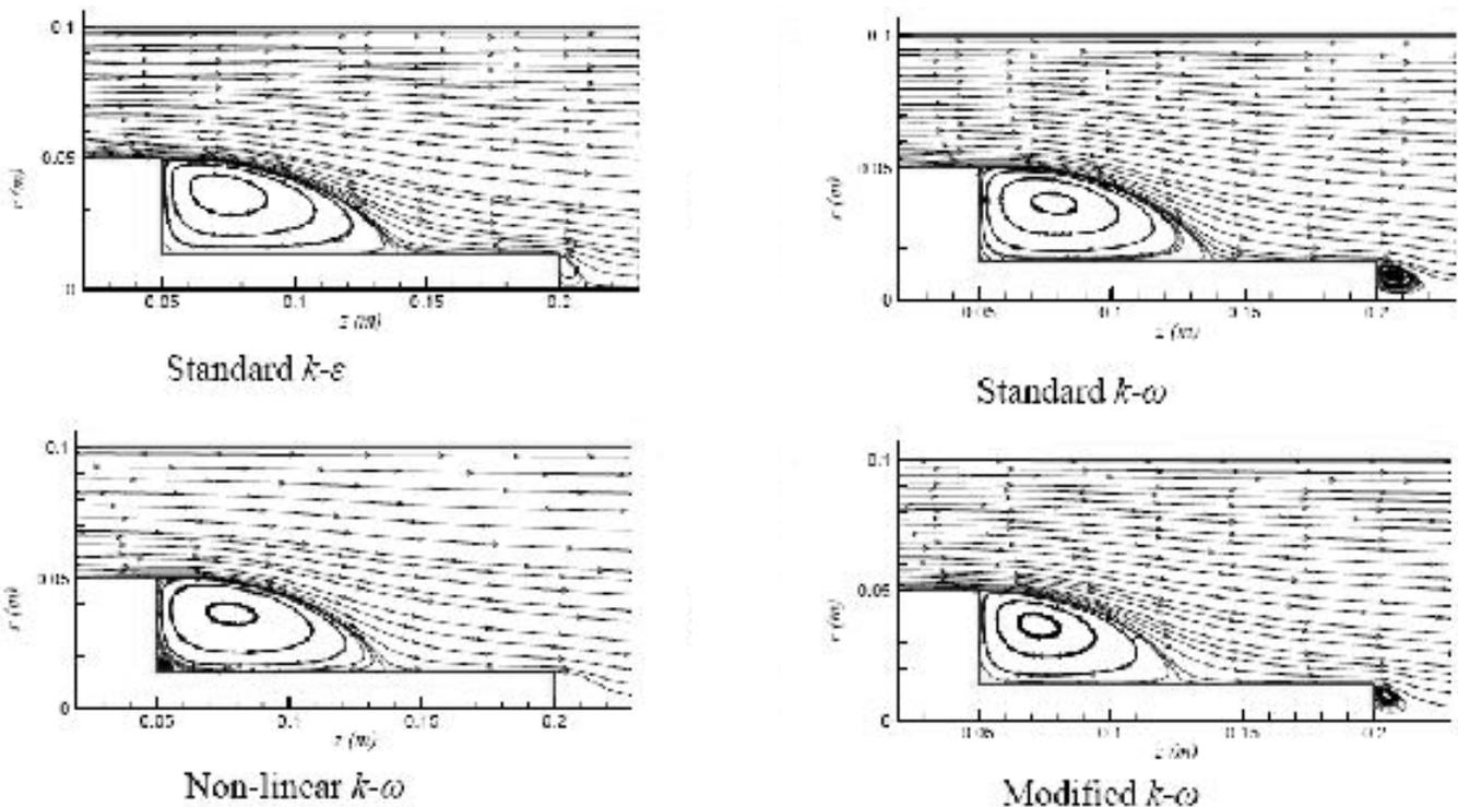
Figure 6. streamline plots for forebody-spindle combination alone.
