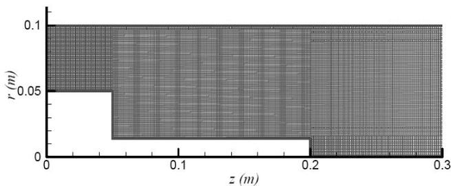
Figure 3. A typical computational grid for standard model.
