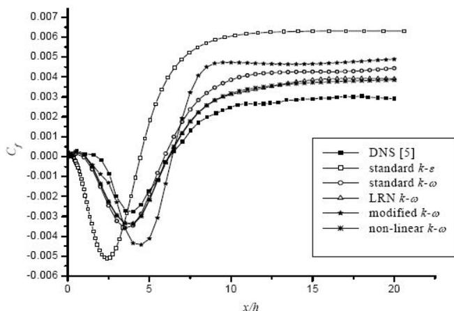
(a) Comparison of skin friction coefficient along the bottom wall of the BFS
