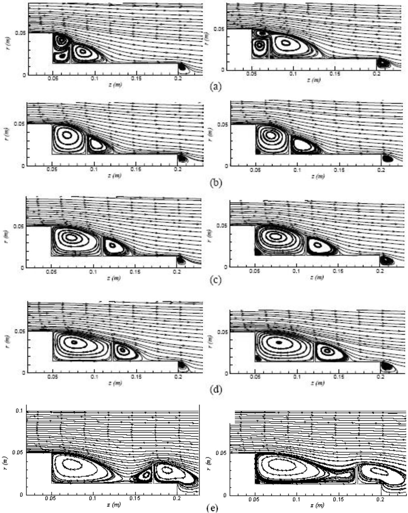
Figure 9. Comparison of streamlines obtained using modified  $k-\omega$  and non-linear  $k-\omega$  for forebody-spindle-disk combination for various disk locations.  $Z_c/D_0 =$  (a) 0.2, (b) 0.4, (c) 0.6, (d) 0.7 and (e) 1.2.
