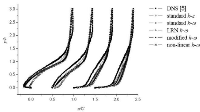
(b) Comparison of normalised mean velocity profiles at  $x/h = 4, 6, 10$  and  $15$
