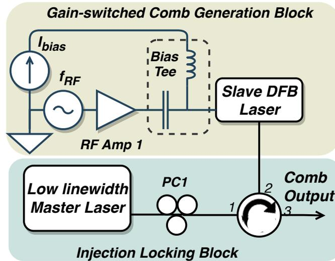
Fig. 2. Schematic of the gain-switched comb generation.
