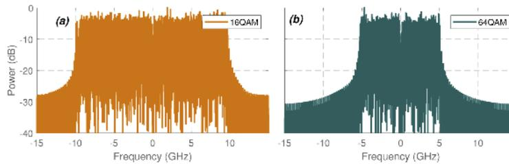
**Fig. 6.** Baseband spectrum of the generated (a) 16QAM CO-OFDM signal (19 GHz bandwidth) and (b) 64QAM CO-OFDM signal (10 GHz bandwidth).
