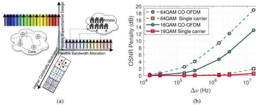
**Fig. 1.** (a) Multi-dimensional agility of coherent optical OFDM (b) OSNR penalty evaluated for a BER of  $1 \times 10^{-3}$  at various linewidth for systems employing 16/64QAM CO-OFDM and Nyquist shaped single carrier modulation with baseband sampling rate/symbol rate of 30 GS/s.
