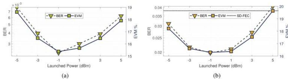
Fig. 8. Launched power optimization performed for 8 channel 16QAM CO-OFDM transmission showing BER and EVM vs launched power (b) Launched power optimization performed for 8 channel 32QAM CO-OFDM transmission showing BER and EVM vs launched power.
