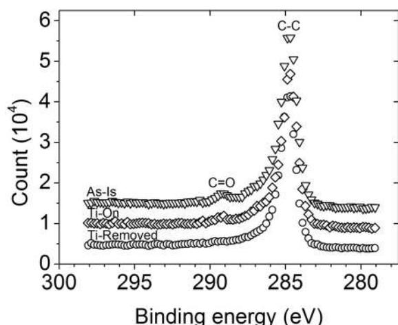
FIG. 3. The C1s XPS spectra of the as-is, Ti-On, and Ti-removed samples (triangles, diamonds, and circles, respectively). The C=O peak located at 289 eV is completely removed following the Ti etching indicating complete removal of the PMMA.
