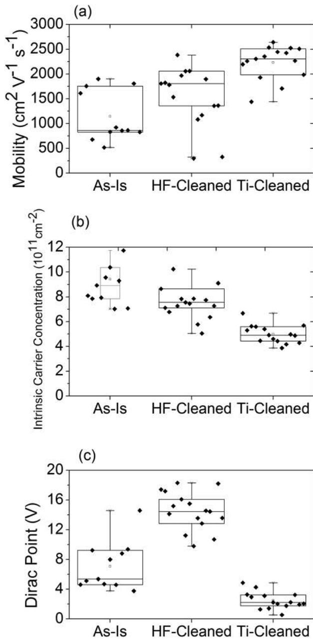
FIG. 1. (a) Mobility measurements of the as-is, HF-cleaned, and Ti-cleaned devices. Ti cleaning results in the highest mobility. (b) Intrinsic or impurity carrier concentration measurements. The Ti cleaning results in a significant improvement. (c) Minimum conductance point measurements. The Ti-Clean devices shift towards the intrinsic point of graphene while the HF cleaning shifts away from the intrinsic point of 0 V.
