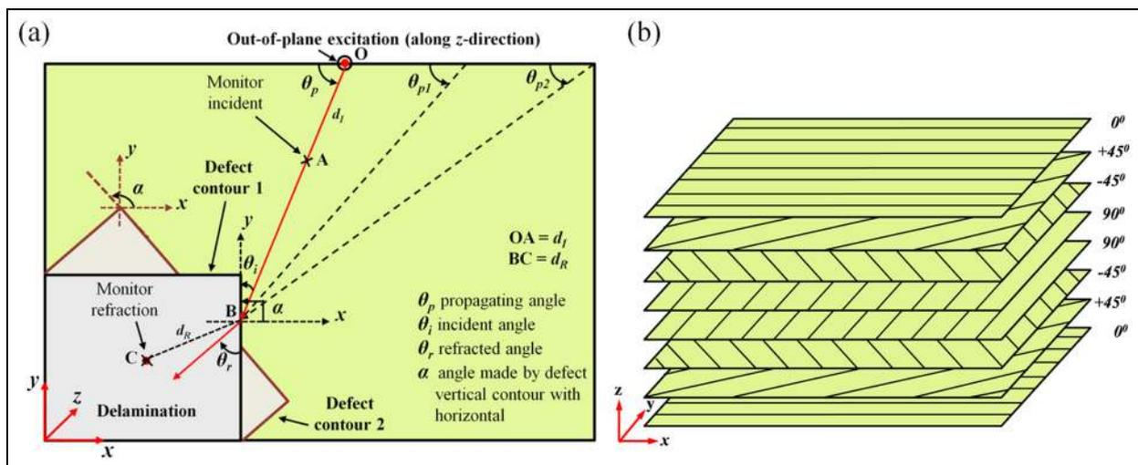
**Figure 4.** (a) Composite laminates with defect orientation and position and (b) ply layups.
