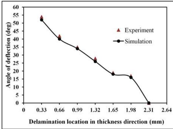
**Figure 7.** Variation of angle of wave deflection with delamination location in thickness direction.
