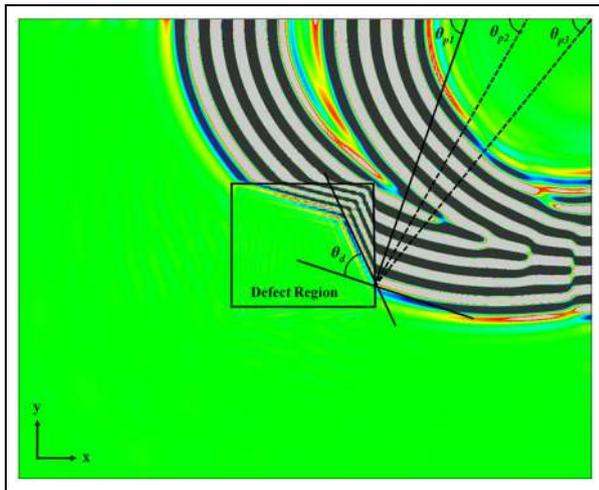
**Figure 10.** Displacement contour showing deflection of  $A_0$  mode in defective zone (FE simulation).
