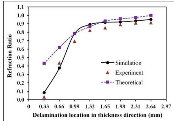
**Figure 8.** Variation of refraction ratio with through-thickness delamination location.
