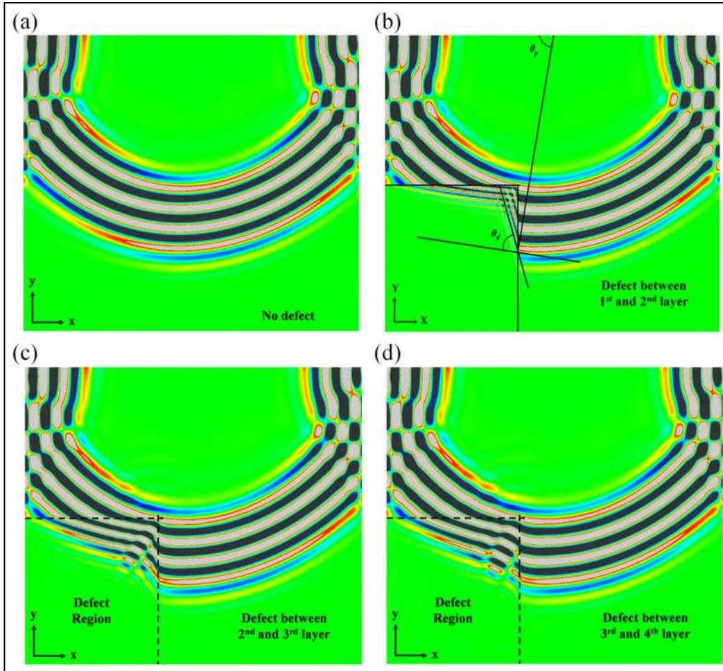
**Figure 6.** Contours of displacement magnitude as obtained from FE simulations at  $96 \mu\text{s}$  for  $A_0$  mode interaction with defects between different layers: (a) no defect, (b) one and two, (c) two and three and (d) three and four.
