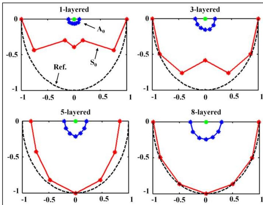
**Figure 9.** Normalized velocity curves for different layered combinations.
