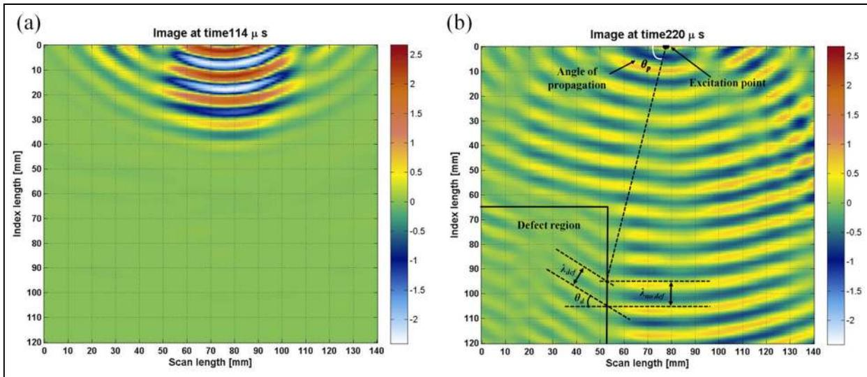
**Figure 5.** Experimental results showing the  $A_0$  mode propagation and interaction with delamination between third and fourth laminas at different times: (a)  $114 \mu\text{s}$  and (b)  $220 \mu\text{s}$ .
