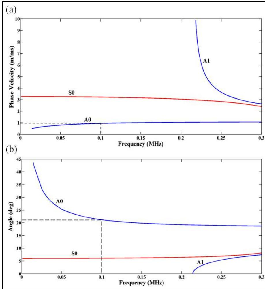
Figure 1. Plot showing (a) phase velocity dispersion curve and (b) incident angle dispersion curve.
