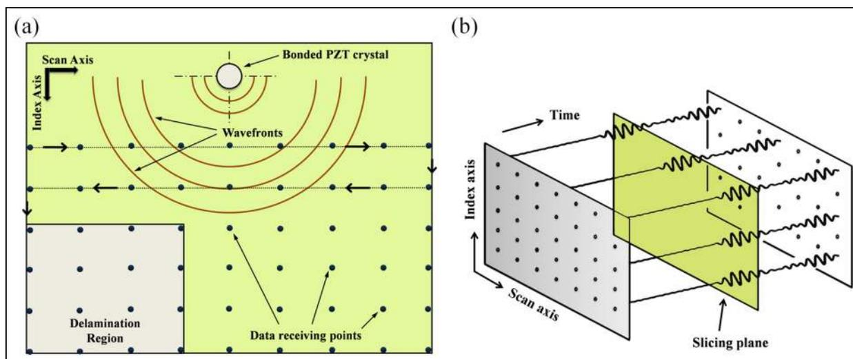
**Figure 3.** (a) A-scan receiving points and (b) displacement field at a particular time instant.
