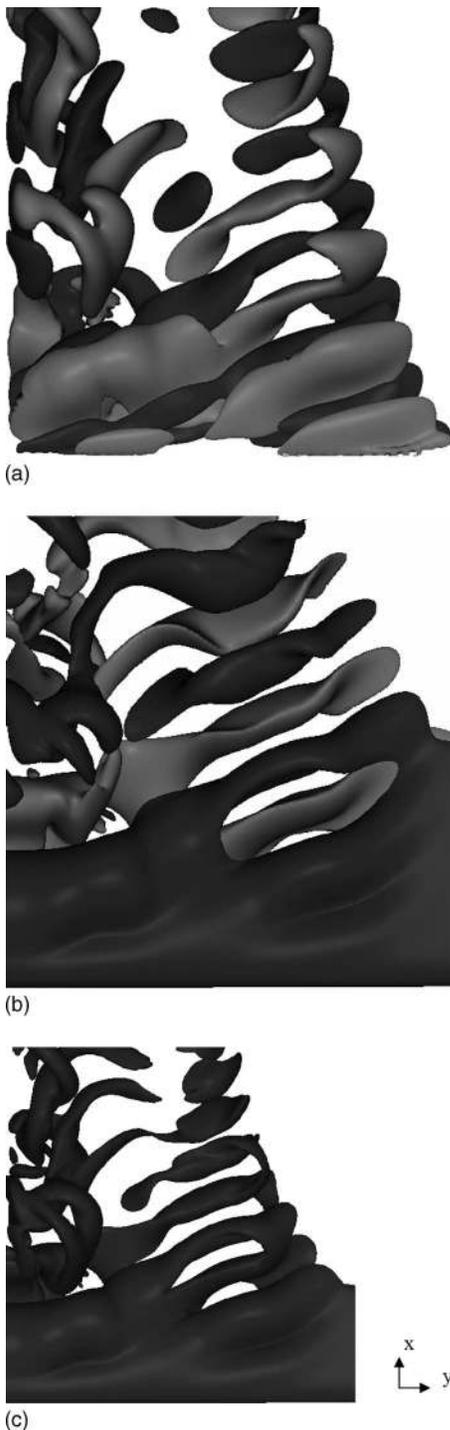
FIG. 16. (a) 3D isosurface plot of streamwise vorticity at time  $t=360d_2/U_0$ . The plate is at the bottom of these figures with the wide end to the left and the flow is upwards. White:  $\omega_x v/U_0^2=-0.004$ ; black:  $\omega_x v/U_0^2=+0.004$ . (b) Spanwise vorticity, otherwise as in (a). (c) Vorticity magnitude  $|\omega|v^2/U_0^4=5e-5$ , otherwise as in (a).
