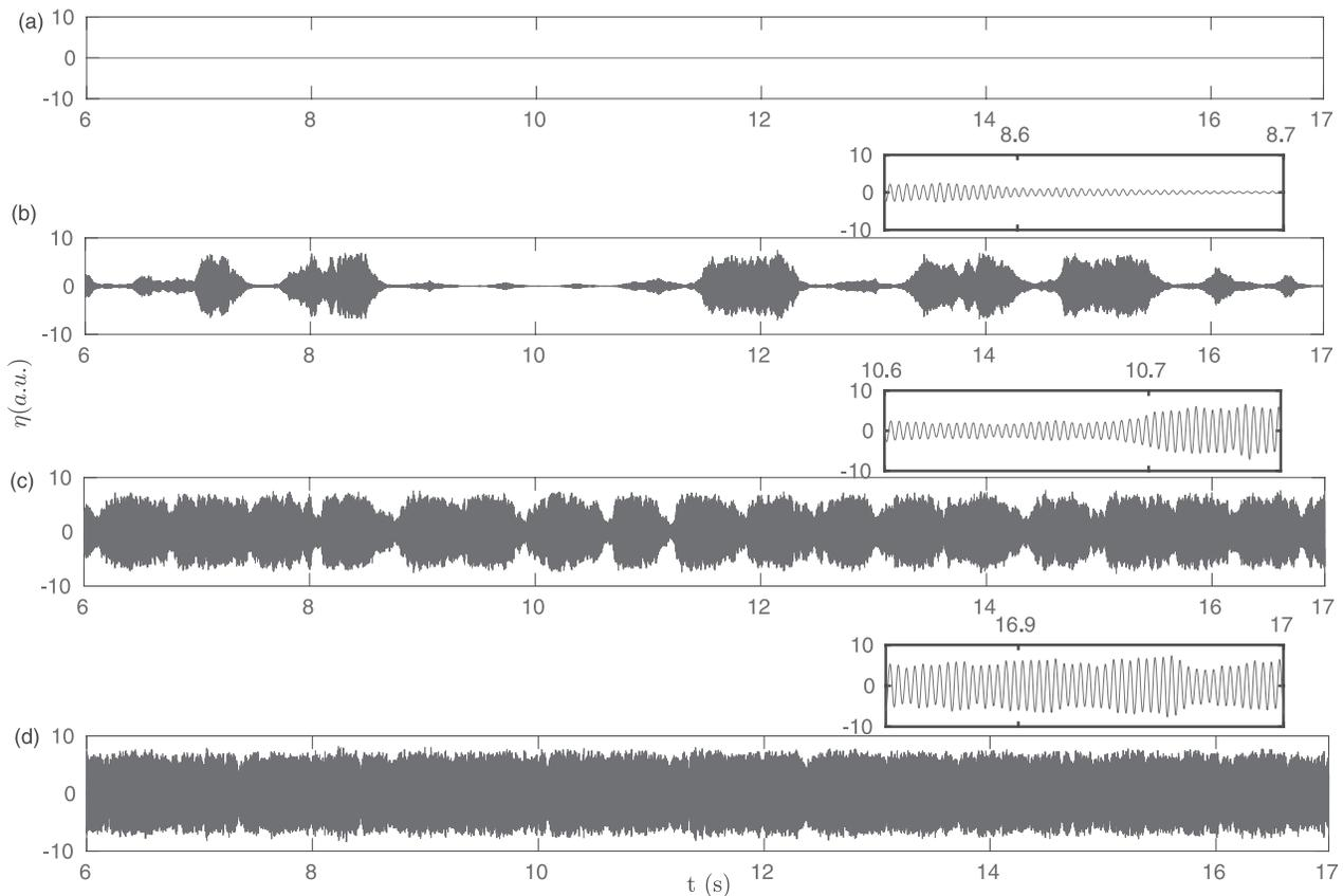
**FIG. 6.** The time series of acoustic pressure fluctuations along with their zoomed insets obtained using the model is shown during (a) stable operation, (b) bursting oscillations, (c) mixed mode oscillations, and (d) limit cycle oscillations. The values of  $\alpha = 58, 52, 37,$  and  $5$  rad/s, respectively.
