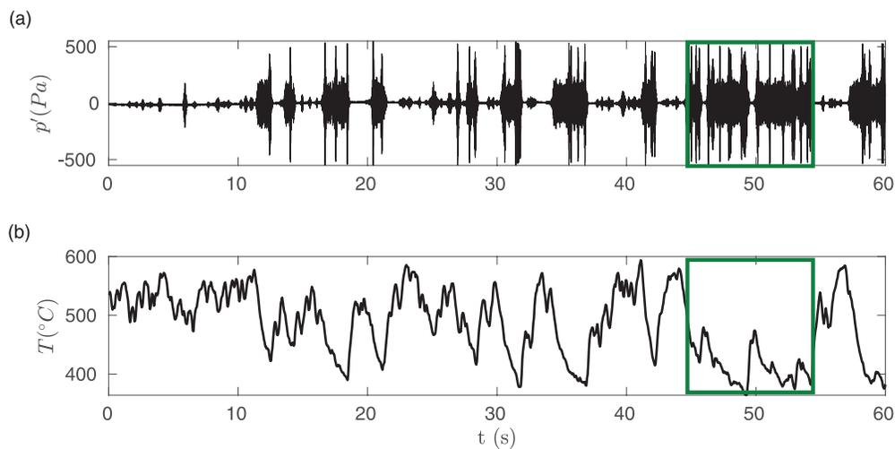
**FIG. 4.** The time series of (a) acoustic pressure oscillations and (b) temperature oscillations obtained simultaneously for a duration of 60 s during bursting oscillations. We conjecture that the simultaneous coexistence of slow-fast time scales gives birth to bursting and mixed mode oscillations.
