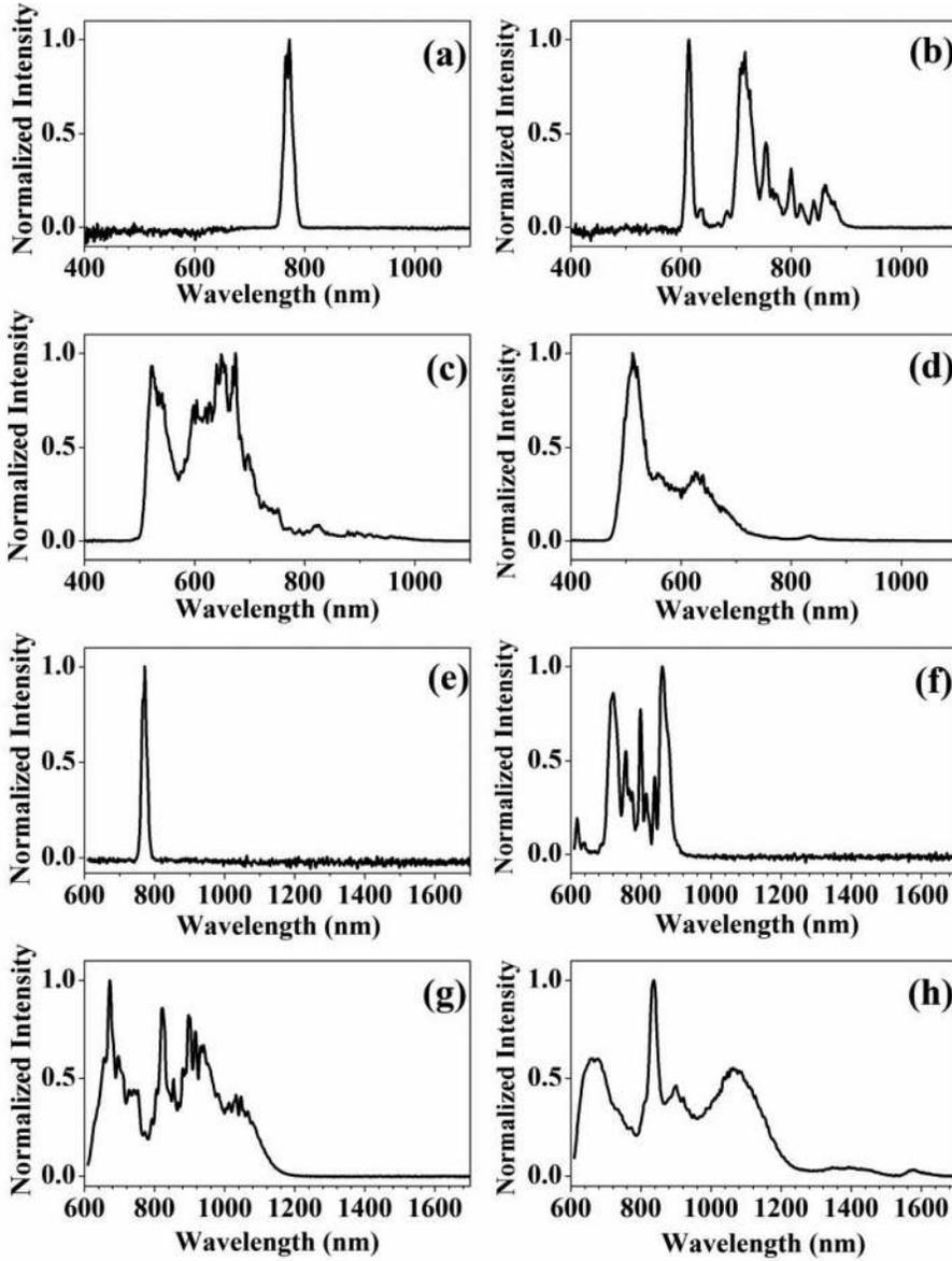
FIG. 3. Femtosecond SC spectra (normalised to unity) from PCF at various values of input power [(a)  $<10$  mW, (b) 30 mW, (c) 170 mW, and (d) 266 mW] recorded with HR2000 spectrometer. The spectra (e)  $<10$  mW, (f) 30 mW, (g) 170 mW, and (h) 266 mW are recorded with IR spectrometer.
