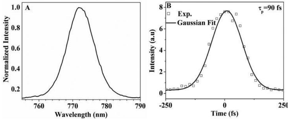
FIG. 1. Spectral (panel A) and temporal (Panel B) profiles of mode-locked pulse.  $\tau_p$  is the pulse width of the laser.
