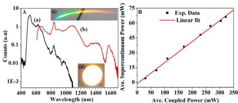
FIG. 4. Full SC spectrum (with y-scale in log) generated from PCF recorded by HR2000 spectrometer (curve (a)) and IR spectrometer (curve (b)). The spectra have been normalized at 663 nm. The inset (bottom) shows the photo of the white light spot and the inset (top) is dispersed photo of the spot with the help of a grating. Panel (b) gives the obtained average SC power with respect to the input power of fundamental beam. Symbols are experimental data and solid line is linear fit.
