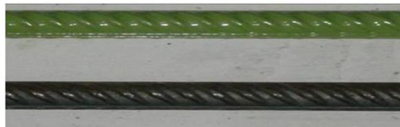
Figure 2. Deformation Pattern of reinforcing bars.
