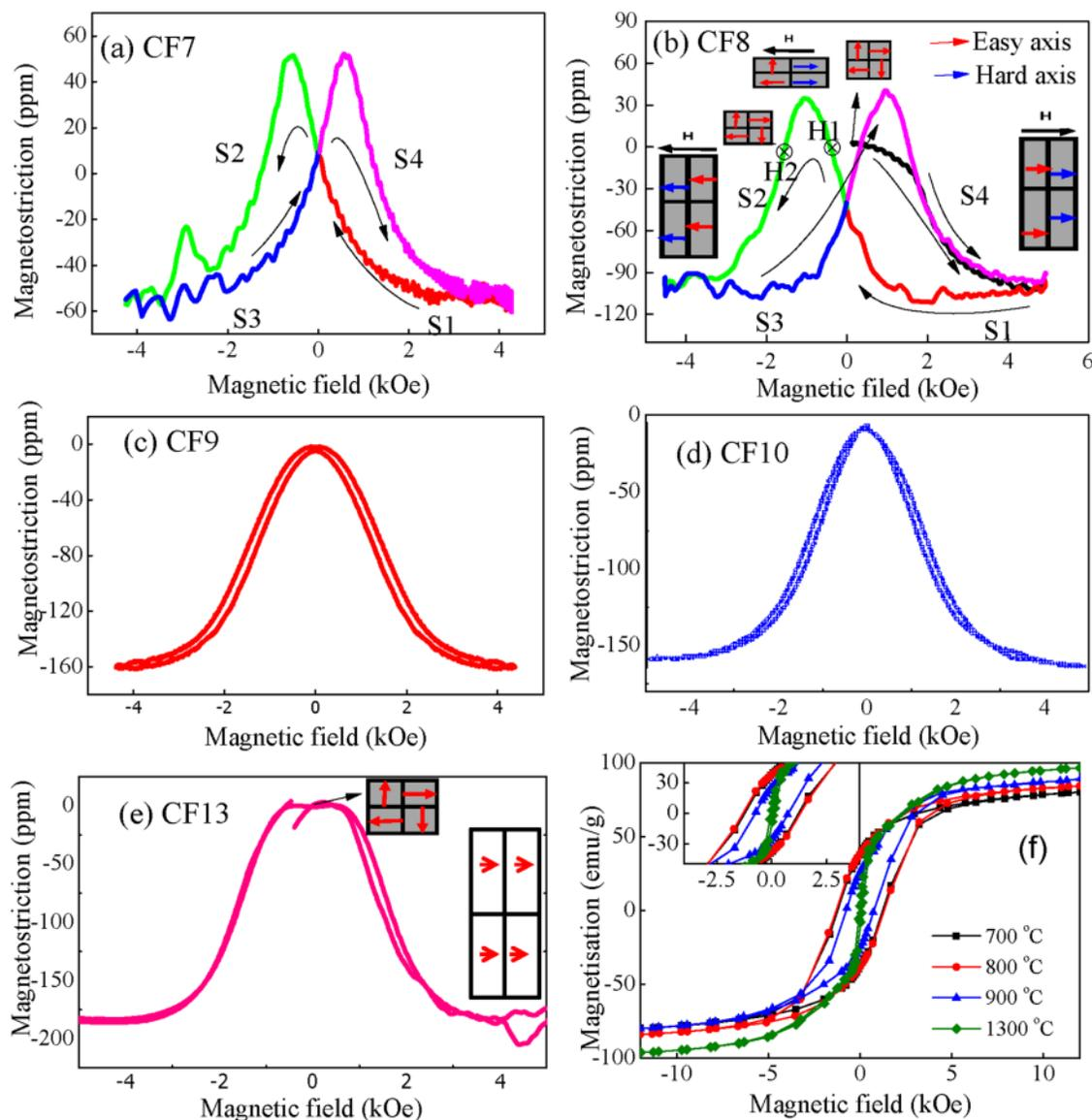
FIG. 4. Magnetostriction curves of samples sintered at (a) 700 °C, (b) 800 °C, (c) 900 °C, (d) 1000 °C, (e) 1300 °C, and (f) M-H loops of sintered samples.
