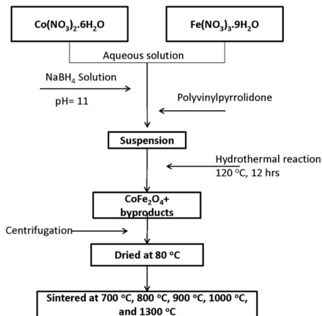
FIG. 1. Flow chart of hydrothermal synthesis procedure.
