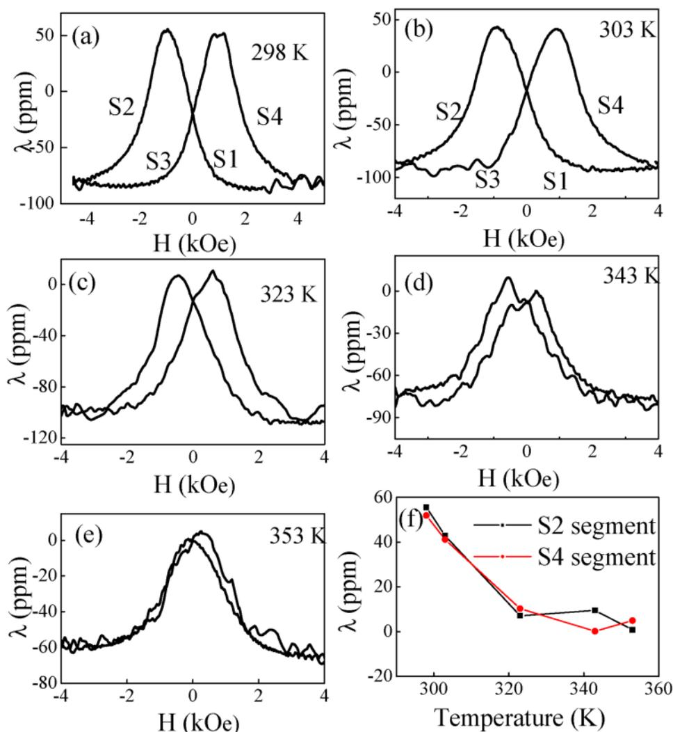
**FIG. 6.** (a)–(e) Temperature-dependent magnetostriction curves for the CF8 sample and (f) variation of peak magnetostriction of S2 and S4 segments with measurement temperature.
