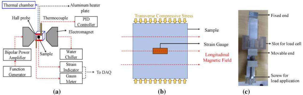
FIG. 2. (a) Schematic of the magnetostriction measurement setup (b) schematic of magnetic field and stress orientations and (c) Photograph of the sample holder for prestress application.
