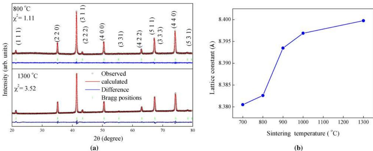
FIG. 3. (a) XRD patterns of sintered samples CF8 and CF13 and (b) lattice constant variation with sintering temperature.
