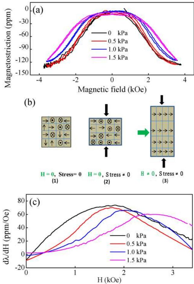
FIG. 7. (a) Magnetostriction curves measured for a CF13 sample at different external compressive stresses, (b) schematic illustration of domain orientation for CF13, and (c) piezomagnetic coefficient at various applied stresses.
