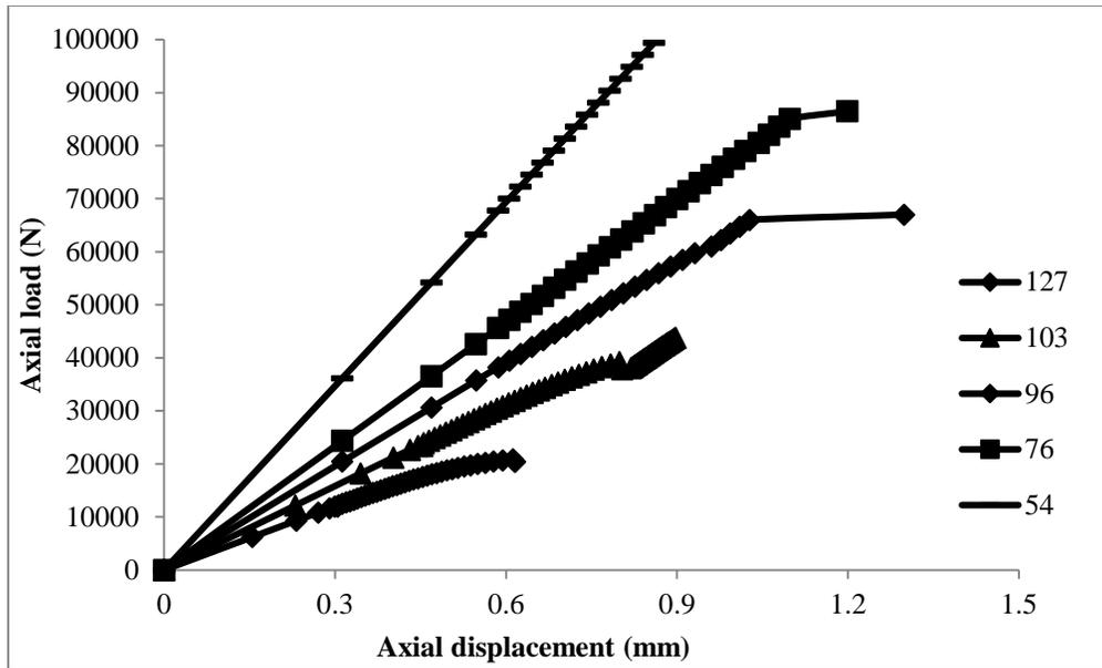
Fig. 5: Load vs axial shortening with varying slenderness ratios.
