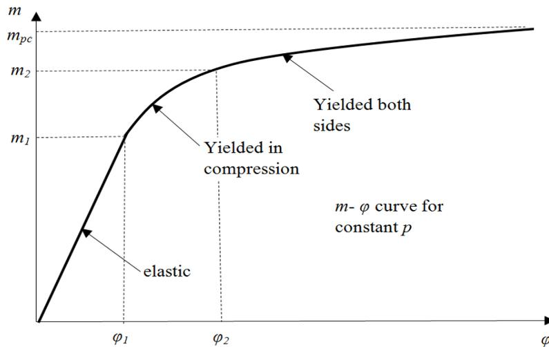
Fig. 3: Moment-curvature-load relationship of imperfect tubular column [3].
