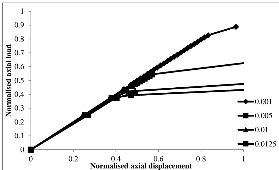
Fig. 4: Load vs axial shortening with varying imperfection.
