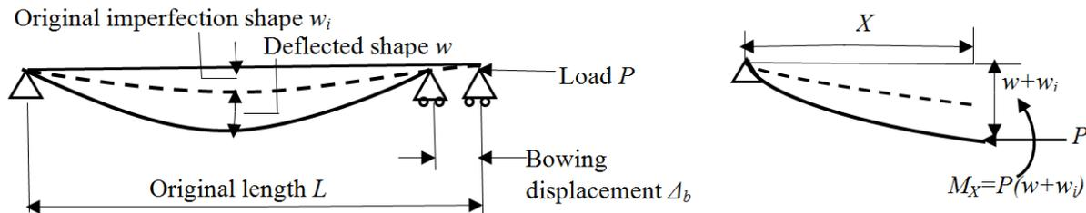
Fig. 1: Buckling in the imperfect column.
