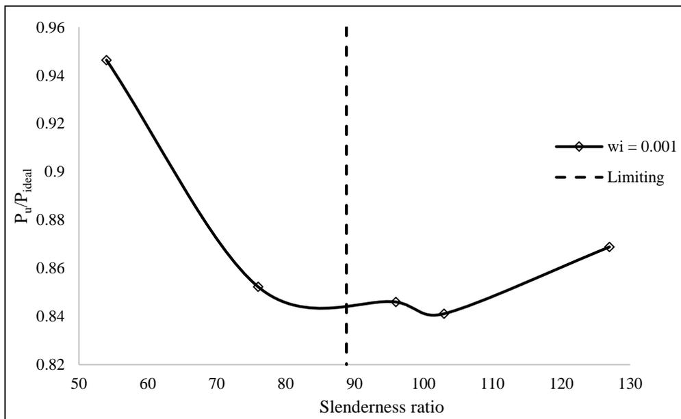
Fig. 6: Ultimate load reductions with slenderness ratio variation.
