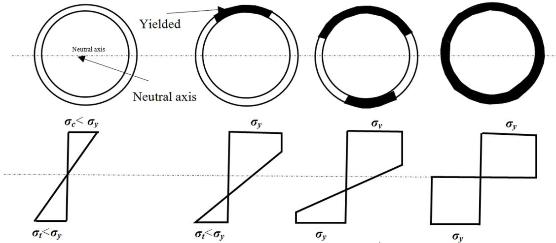
Fig. 2: Cross-section stress distribution.
