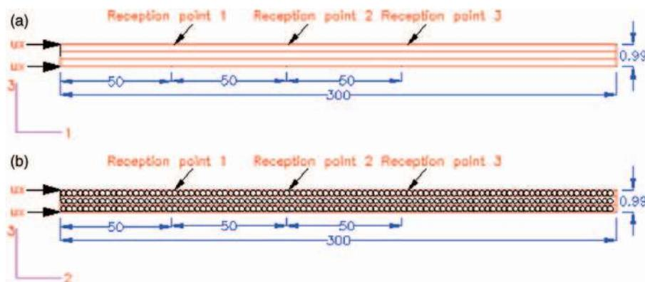
Figure 3. Specification of model used for FE simulations. Excitation of  $S_0$  mode (a) along fibers and (b) across fibers.
