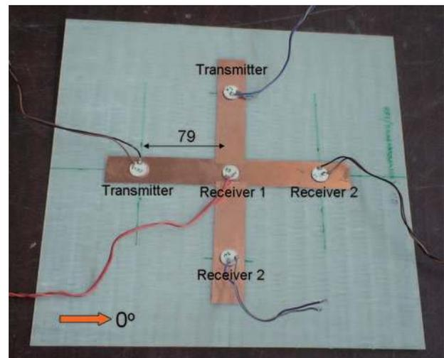
Figure 5. PZT patches bonded on glass/epoxy UD laminate.
