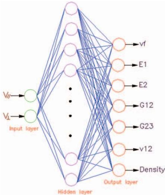
**Figure 1.** Neural network used for predicting elastic properties, fiber volume fraction, and density.
