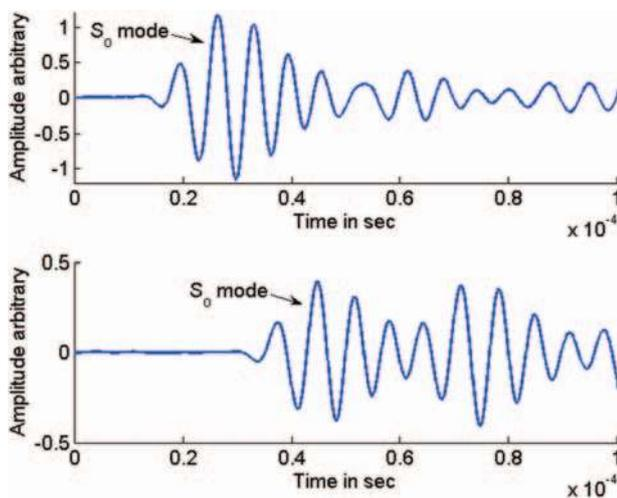
**Figure 6.** A-scans from experiments, taken at (a) “Receiver 1” and (b) “Receiver 2” along fiber direction.
