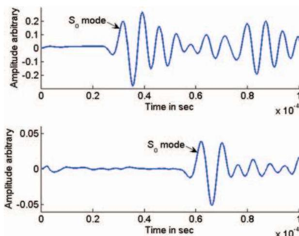
**Figure 7.** A-scans from experiments, taken at (a) “Receiver 1” and (b) “Receiver 2” across fiber direction.
