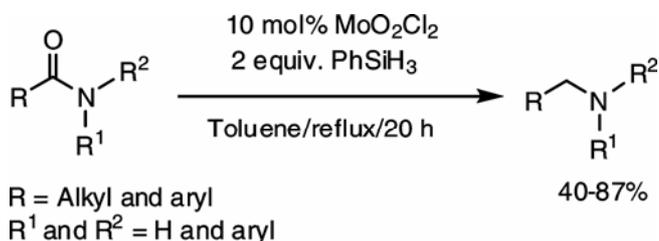
**Scheme 18.** Reduction of amides using silane/ $\text{MoO}_2\text{Cl}_2$ .
