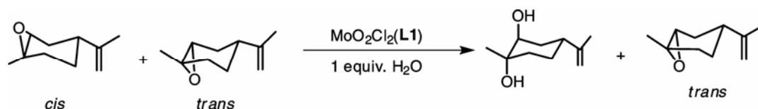
**Scheme 30.** Diastereoselective ring opening of limonene oxide with water using MoO<sub>2</sub>Cl<sub>2</sub> (L1).
