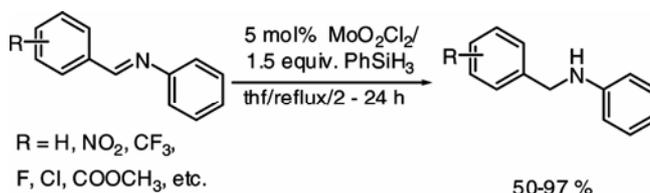
**Scheme 7.** Reduction of various imines using silane/MoO<sub>2</sub>Cl<sub>2</sub>.
