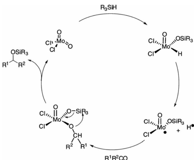
**Figure 4.** Proposed mechanism for MoO<sub>2</sub>Cl<sub>2</sub> catalysed hydrosilylation reactions.
