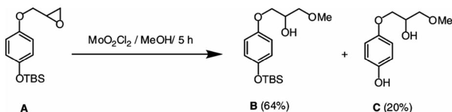
**Scheme 27.** Methanolysis of *tert*-butyldimethylsilyl (TBS) protected epoxide.
