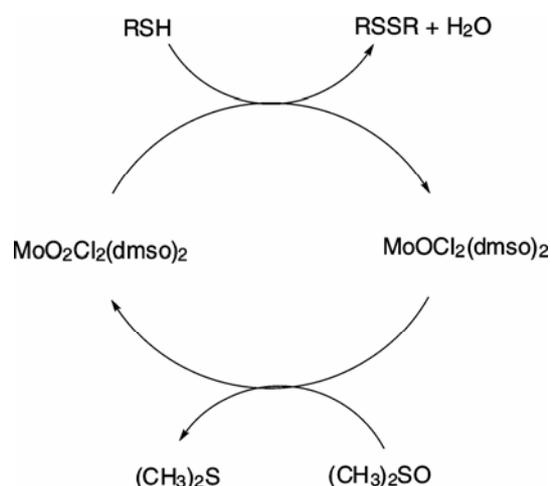
**Figure 8.** Proposed mechanism for oxidation of thiols by MoO<sub>2</sub>Cl<sub>2</sub>(dmsO)<sub>2</sub>.
