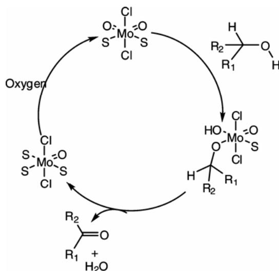
**Figure 9.** Proposed mechanism for  $\text{MoO}_2\text{Cl}_2$ ( $\text{dmsO}$ )<sub>2</sub> catalysed alcohol oxidation. (S = solvent).
