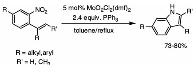
**Scheme 20.** Synthesis of indoles by reductive cyclization of nitroaromatics.
