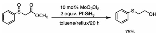
**Scheme 17.** Reduction of methyl-(phenylsulfinyl)acetate.
