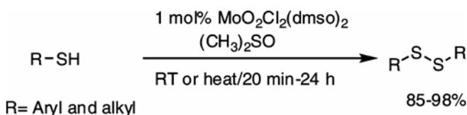
**Scheme 22.** Oxidation of thiols to disulfides.
