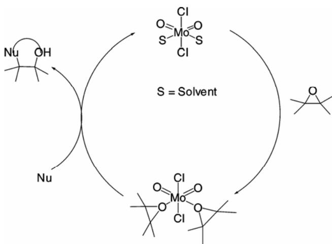
**Figure 10.** Proposed mechanism for epoxide ring opening reaction.
