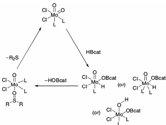
**Figure 5.** Proposed mechanism for the reduction of sulfoxides using MoO<sub>2</sub>Cl<sub>2</sub>/borane.
