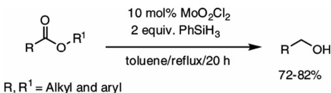
**Scheme 15.** Reduction of esters using silane/ $\text{MoO}_2\text{Cl}_2$ .
