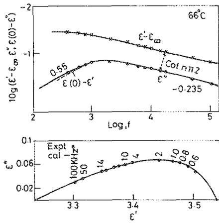
FIG. 3. Dielectric behavior of one polyether-urethane sample. (a) Double logarithmic representation of the real and imaginary parts of  $\epsilon^* - \epsilon_\infty$  with frequency. (b) Complex plane representation for the same.
