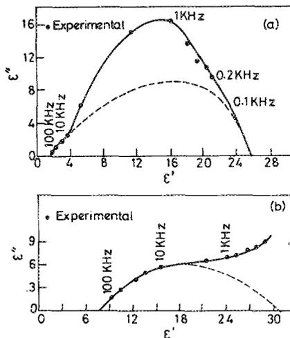
FIG. 1. (a) The complex plane representation of the dielectric behavior of Ni-Zn 1 at 50 °C. (b) The complex plane representation of the dielectric behavior of Ni-Zn 3 at 50 °C.
