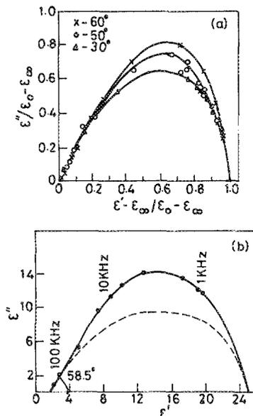
FIG. 2. (a) The complex plane representation of the dielectric behavior of Ni-Zn-Mn 1 at 50 °C. (b) Temperature variation of the dielectric behavior of Ni-Zn 1 shown as a normalized complex plane plot.
