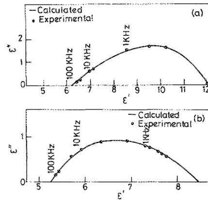
FIG. 4. (a) Complex plane representation of the dielectric behavior of wax-Ni-Zn 1 at room temperature. (b) Complex plane representation of the dielectric behavior of wax-Ni-Zn 3 at room temperature.
