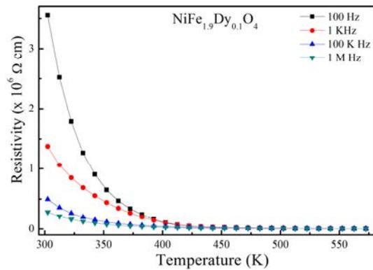
**Figure 3:** Plot of resistivity vs temperature of  $\text{NiFe}_{1.9}\text{Dy}_{0.1}\text{O}_4$  for different frequencies
