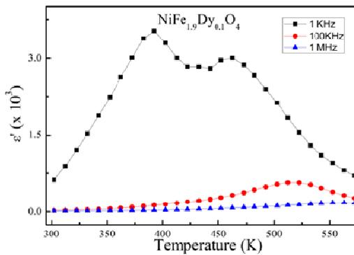
**Figure 2** Plot of permittivity vs temperature of  $\text{NiFe}_{1.9}\text{Dy}_{0.1}\text{O}_4$  for different frequencies
