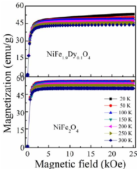
**Figure 4:** Magnetization curves of  $\text{NiFe}_{2-x}\text{Dy}_x\text{O}_4$  ( $x = 0, 0.1$ ) at different temperatures
