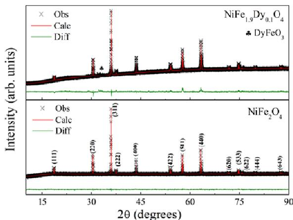
**Figure 1:** Rietveld refined XRD patterns of  $\text{NiFe}_{2-x}\text{Dy}_x\text{O}_4$  ( $x = 0, 0.1$ )
