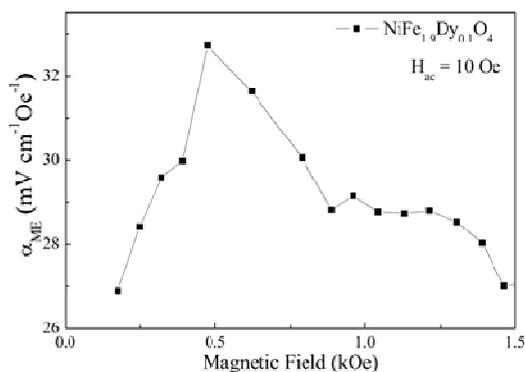
**Figure 6:** Plot of  $\alpha_{\text{ME}}$  vs magnetic field at room temperature  $\text{NiFe}_{1.9}\text{Dy}_{0.1}\text{O}_4$
