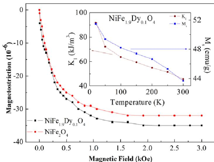
**Figure 5:** Room temperature magnetostriction of  $\text{NiFe}_{2-x}\text{Dy}_x\text{O}_4$  ( $x = 0, 0.1$ ). Inset: Temperature dependence of  $M_s$  and  $K_1$  of  $\text{NiFe}_{2-x}\text{Dy}_x\text{O}_4$  ( $x = 0, 0.1$ )
