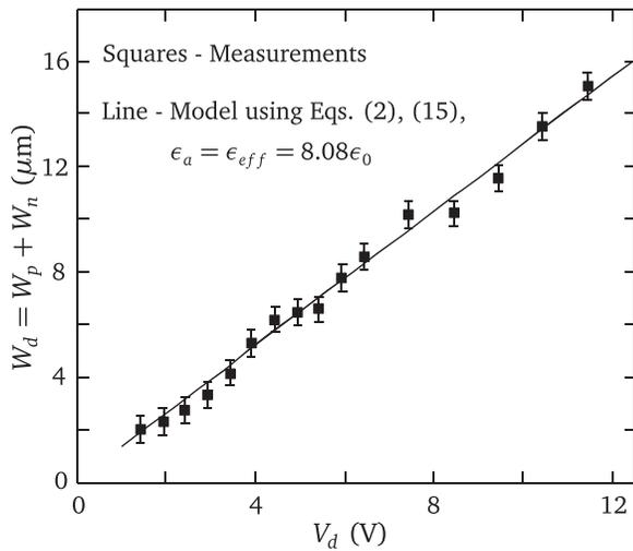
FIG. 6. Comparison between the measured<sup>27</sup> and modelled depletion width versus potential drop behaviors in a reverse biased lateral  $p$ - $n$  junction realized in a 10 nm InGaAs nanofilm stacked between the ambients of 650 nm GaAs buffer and 175 nm AlGaAs/GaAs-AlAs/AlGaAs multilayer.
