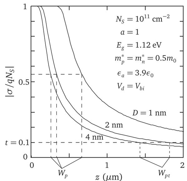
FIG. 5. The simulated  $p$ -side space-charge distribution under equilibrium as a function of distance from the junction for films of different thicknesses having quantum confinement effects; the depletion and space-charge tail widths are indicated.
