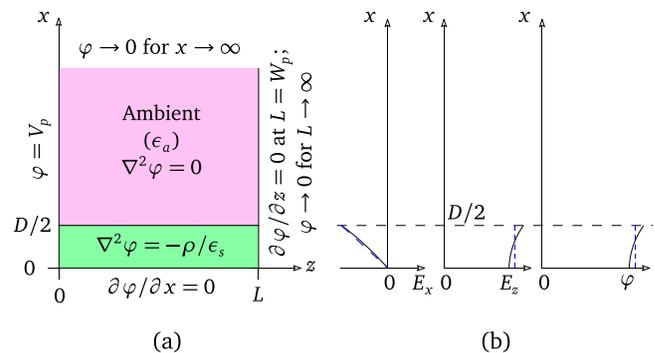
FIG. 2. (a) The governing equations and boundary conditions for the upper half cross-section of the *p*-side of the nanofilm junction shown in Fig. 1(b);  $\epsilon_1 = \epsilon_2 = \epsilon_a$  is assumed. (b) Variations of actual (solid lines) and approximated (dashed lines)  $E_x$ ,  $E_z$ , and  $\varphi$  over film thickness ( $x \leq D/2$ ); see text for the details of approximations.
