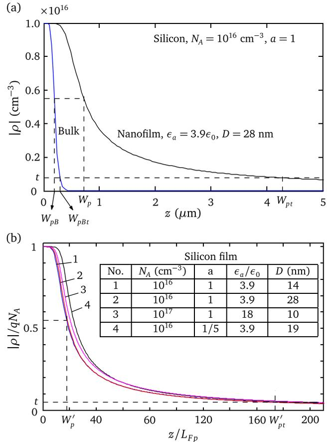
FIG. 4. The simulated  $p$ -side space-charge distribution under equilibrium as a function of distance from the junction; the depletion widths and space-charge tails are indicated. (a) Distributions in bulk and nanofilm junctions. (b) Normalized form of the distributions in sheet-like films illustrating the utility of screening length  $L_{Fp}$ ;  $W'_p$  and  $W'_{pt}$  are indicated for curve 1.
