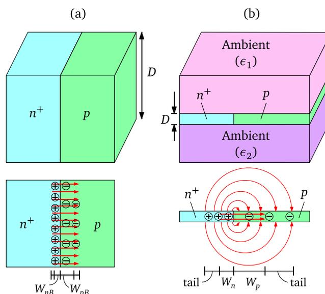
FIG. 1. Space-charge and electric field lines in (a) bulk  $p$ - $n$  junction, and (b) lateral  $p$ - $n$  junction in a nanofilm. The space-charge tails beyond the depletion width are also shown; these are much longer in (b) than in (a). In (b), the field lines correspond to  $\epsilon_1 = \epsilon_2$ . Diagrams are not to scale.
