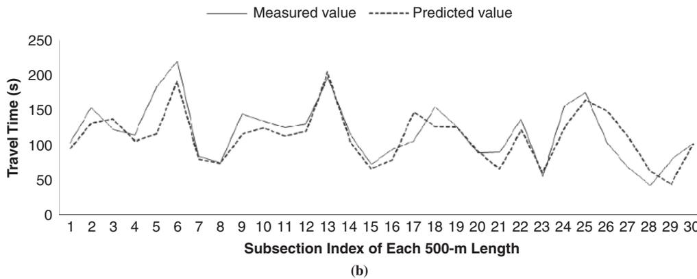
FIGURE 4 Actual and predicted travel times for sample trips over 500-m subsections on (a) Route 19B (MAPE = 13.38) and (b) Route 5C (MAPE = 17.33).
