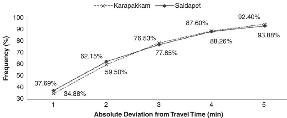
FIGURE 6 Results of predicted arrival time deviation at selected bus stops.
