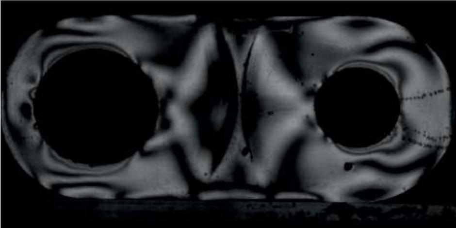
Fig.2 Fringes observed in the stress frozen model
