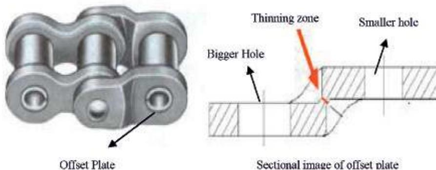
Fig.1A complex shape chain plate
