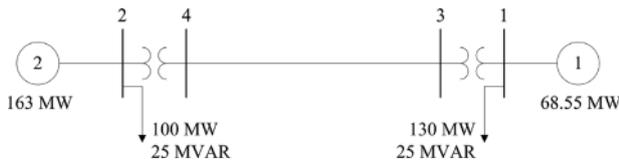
**Figure 5** 2 generator 4 bus test system
