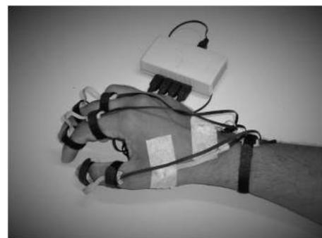
FIG. 3. i-Glove designed for hand rehabilitation/assessment.
