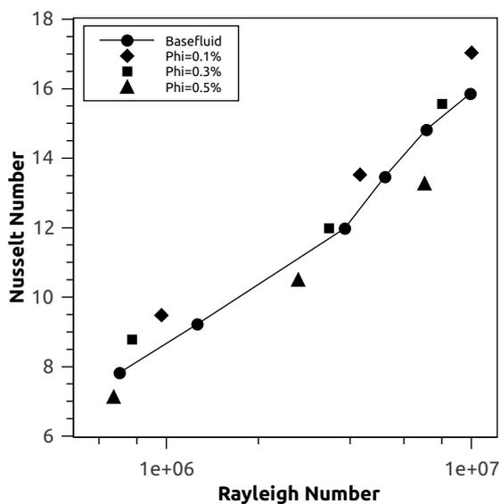
**Figure 10.** Nu vs Ra for MWCNT/Water nanofluid for different  $\phi$ .
