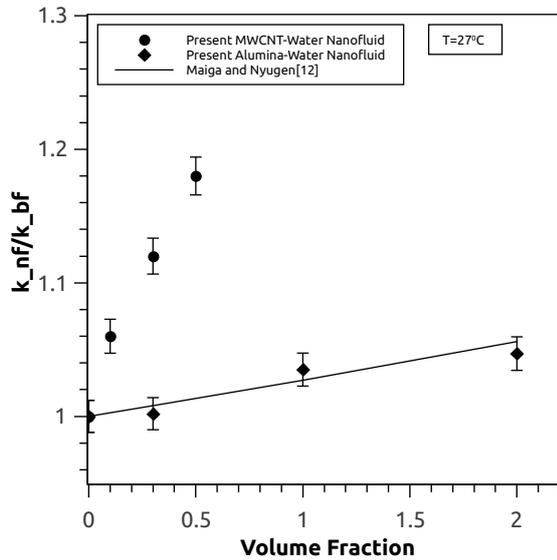
**Figure 5.** Variation of Thermal Conductivity with Volume Fraction.
