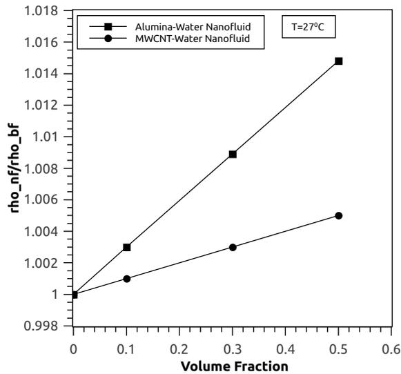
**Figure 7.** Variation of Effective Density of Nanofluid with Volume Fraction.
