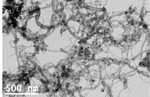
**Figure 4.** TEM image of MWCNT nanoparticle.
