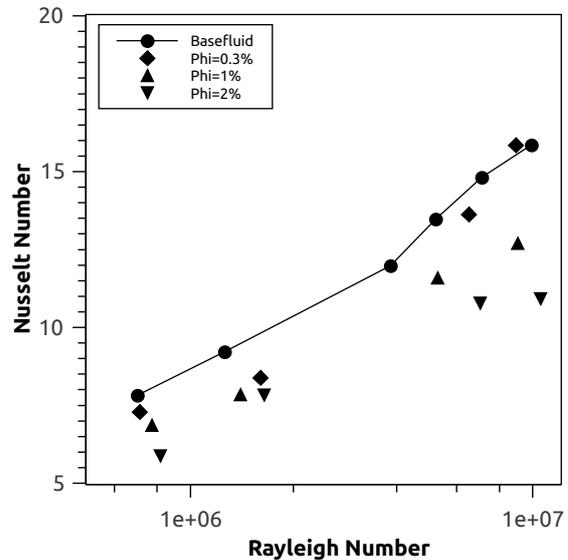
**Figure 9.** Nu vs Ra for  $Al_2O_3$ /Water nanofluid for different  $\phi$ .
