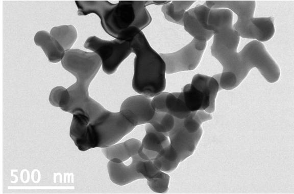
**Figure 3.** TEM image of Alumina nanoparticle.
