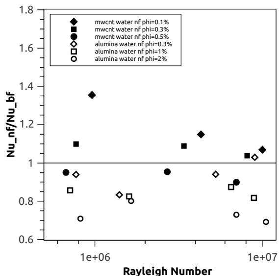
**Figure 11.**  $Nu_{nf}/Nu_{bf}$  vs Ra for different nanofluid
