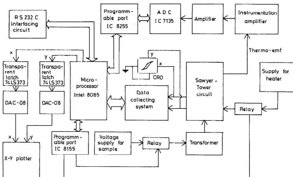
FIG. 1. Block diagram of the automated hysteresis loop tracer.
