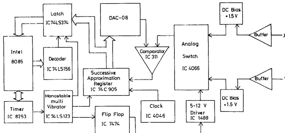
FIG. 3. Block diagram of the ADC used for collecting the hysteresis loop data.
