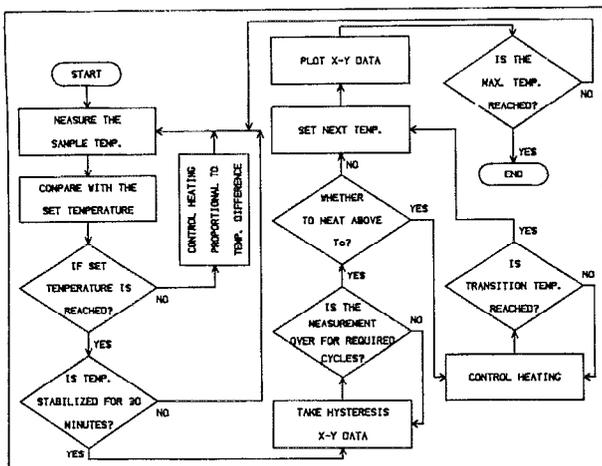
FIG. 2. Flowchart of the overall functioning of the measurement setup.
