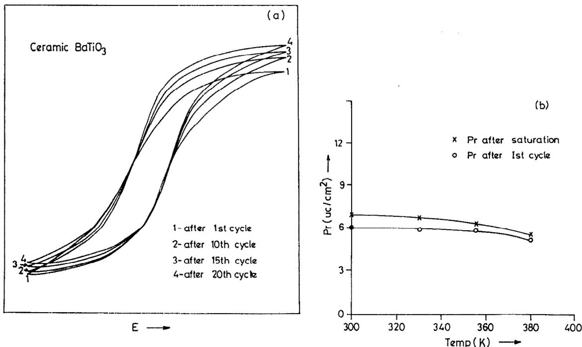
FIG. 4. (a) Variation of hysteresis loop with number of applied field cycles. (b) Variation of remanent polarization with temperature for the different number of cycles of applied field.
