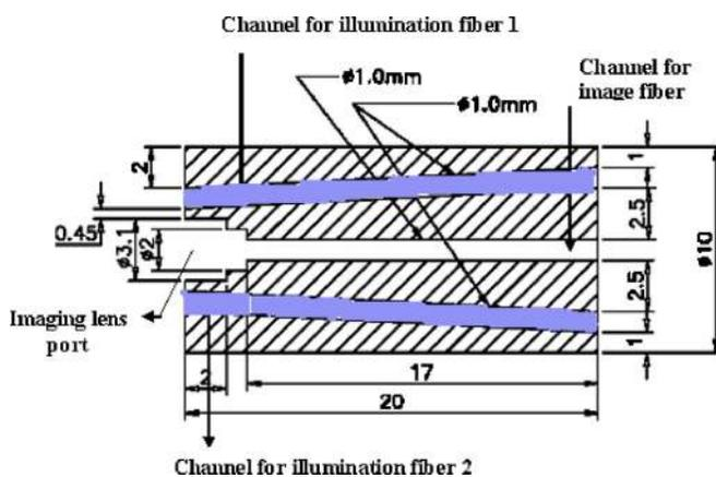
FIG. 2. Dimensions of the endoscope probe distal end.
