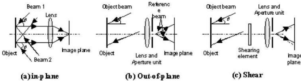
FIG. 4. Schematic diagram showing the illumination directions, illumination angle, and viewing directions for three configurations: (a) in-plane, (b) out-of-plane, and (c) shear configurations.
