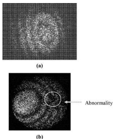
FIG. 13. Out-of-plane fringes obtained using the endoscope system: (a) fringes obtained from normal colon phantom model and (b) fringes obtained from abnormal colon phantom model.
