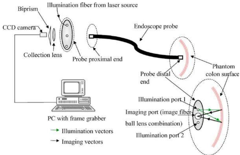
FIG. 10. Schematic diagram of the endoscope system—shear configuration.
