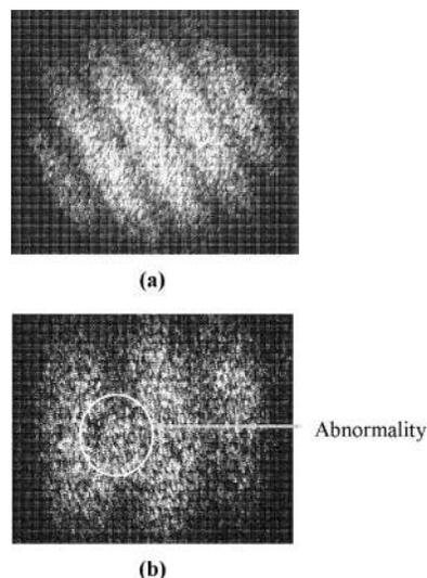
FIG. 12. In-plane fringes obtained using the endoscope system: (a) fringes obtained from normal colon phantom model and (b) fringes obtained from abnormal colon phantom model.
