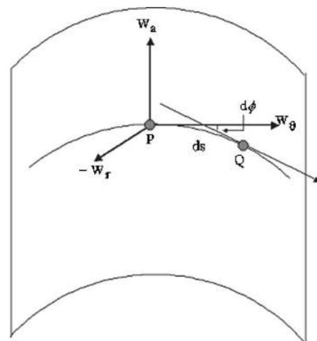
FIG. 5. Different displacement components for a cylindrical specimen ( $ds$ : elemental displacement along the curved surface,  $d\phi$ : angle between the tangents at points  $P$  and  $Q$ ,  $w_r$ : displacement component along radial direction,  $w_\theta$ : displacement component along tangential direction, and  $w_a$ : displacement component along axial direction).
