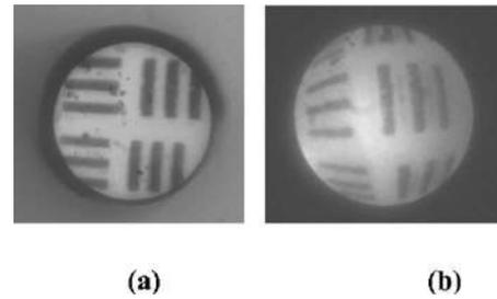
FIG. 3. USAF resolution chart imaged using the proposed system: (a) ball lens of 3 mm diameter and (b) lens with 0.7 mm diameter.
