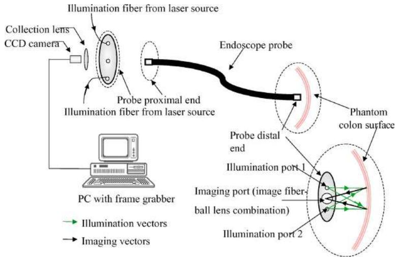
FIG. 6. Schematic diagram of the endoscope system—in-plane configuration.
