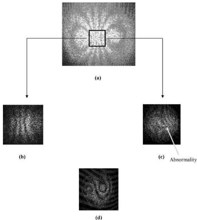
FIG. 14. (a) Fully developed shear fringe obtained from a curved tissue using conventional shear configuration; (b) shear fringes obtained using the endoscope system from normal colon phantom model; (c) shear fringes obtained using the endoscope system from abnormal colon phantom model with a kink at the abnormality site; (d) separate shear fringe system evolved at the abnormality site, captured using the endoscope.
