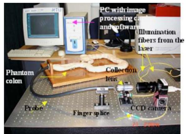
FIG. 7. Developed probe: laboratory prototype—in-plane configuration.
