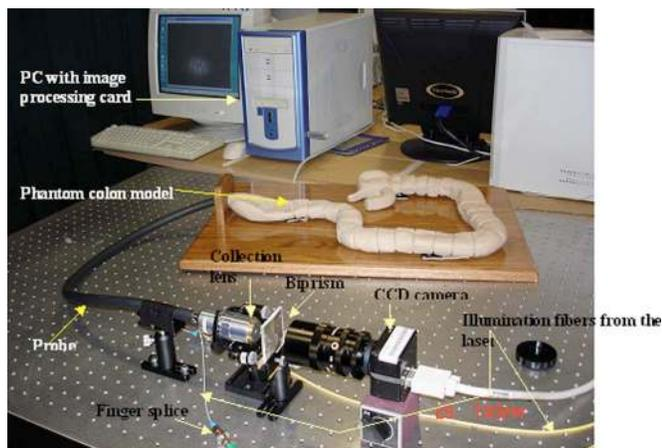
FIG. 11. Developed probe: laboratory prototype—shear configuration.
