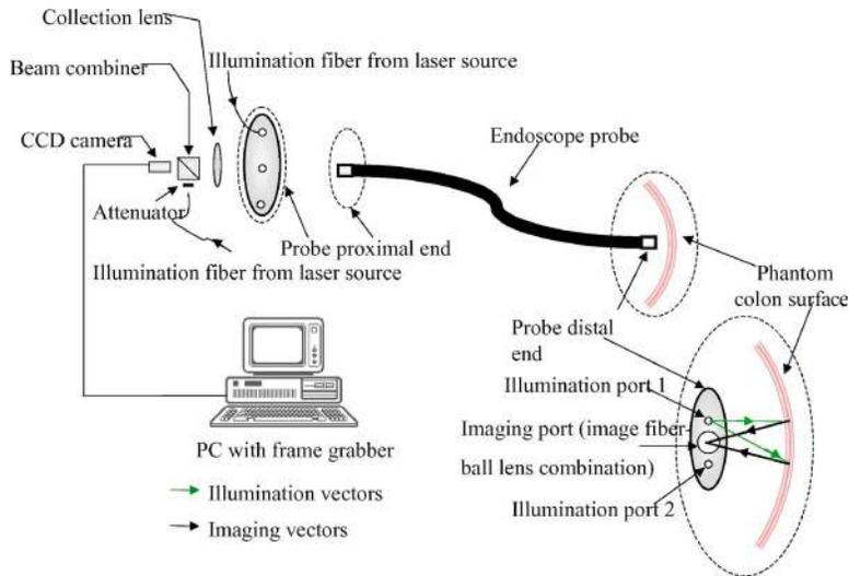
FIG. 8. Schematic diagram of the endoscope system—out-of-plane configuration.
