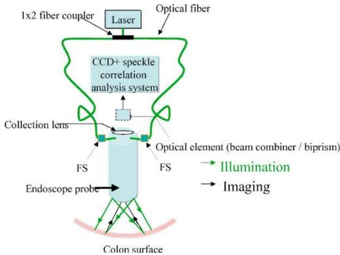
FIG. 1. Schematic of the endoscope system. FS—finger splice (connector).
