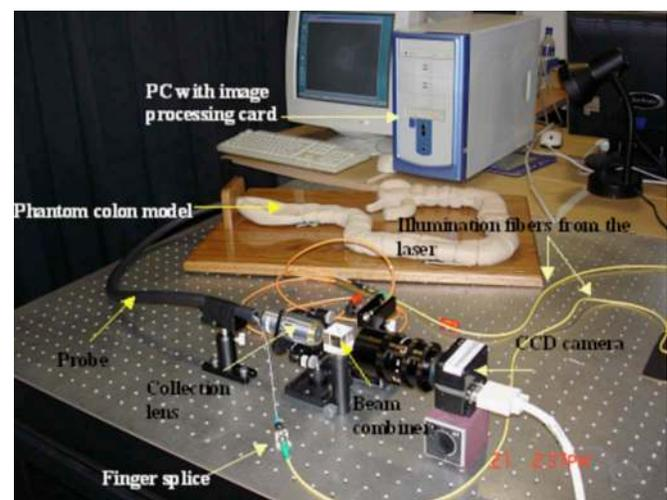
FIG. 9. Developed probe: laboratory prototype—out-of-plane configuration.
