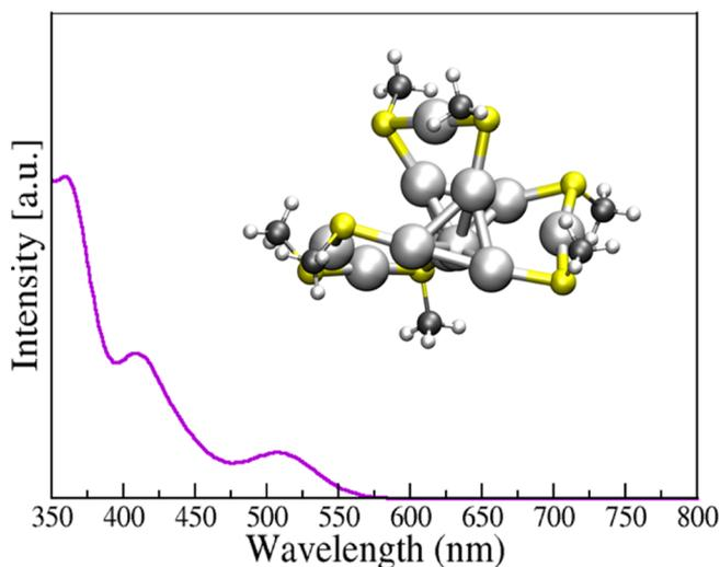
**Figure 7.** Computed optical spectrum of  $\text{Ag}_{11}(\text{SCH}_3)_7$ , structure f. The individual optical lines are broadened with 0.05 eV Gaussians. The structure is shown as an inset.
