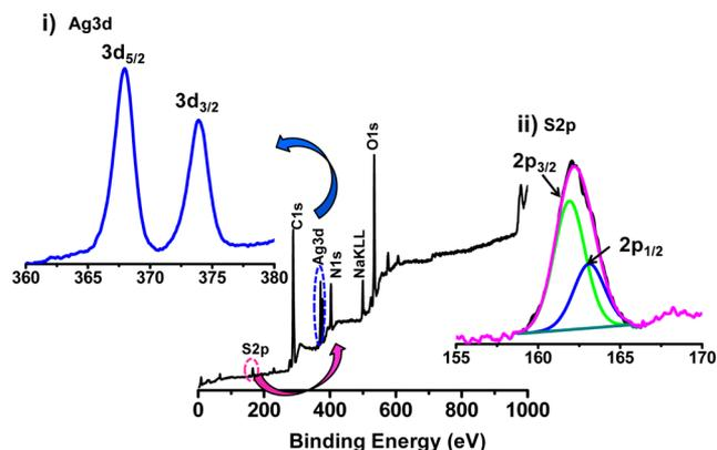
**Figure 3.** XPS survey spectrum of AgSG cluster showing all the expected elements, Ag, S, C, O, N, and Na. Ag 3d and S 2p regions are expanded in (i) and (ii), respectively, showing Ag in  $\text{Ag}^0$  state and sulfur bound to metal.
