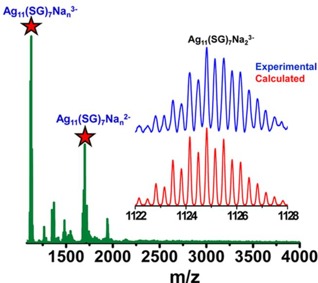
**Figure 4.** ESI MS of the clusters in the negative ion mode showing  $-2$  and  $-3$  charged species along with some thiolates. Main peaks are marked with the \* symbol. Experimental spectrum (blue trace) is in good agreement with the calculated mass spectrum (red trace) of the species as shown in the inset.
