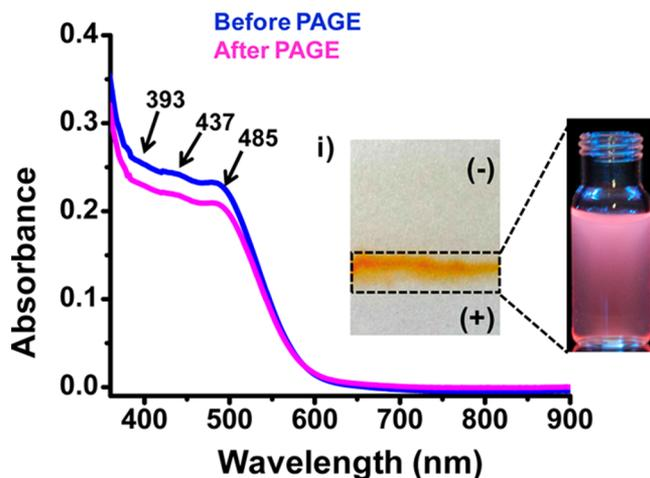
**Figure 2.** UV–vis absorption spectra of silver clusters remain the same before and after PAGE separation. A single band in PAGE (inset (i)) confirms the high purity of the cluster in the as-synthesized form. The band was cut and the cluster was extracted into water. This cluster exhibits red luminescence under UV irradiation (shown on the right).
