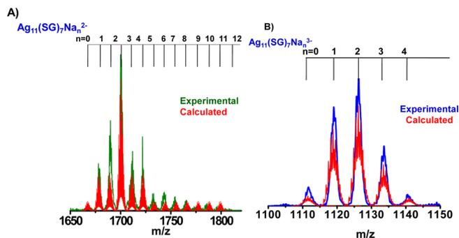
**Figure 5.** Expanded negative mode ESI MS of  $\text{Ag}_{11}(\text{SG})_7$  clusters in  $m/z$  1100–1150 (A) and 1650–1800 (B) ranges. Multiple sodium attachments to glutathione ligand is evident from both the double (A) and triply (B) charged species. Good match of the experimental and calculated mass spectra for  $\text{Ag}_{11}(\text{SG})_7$  with and without sodium adducts is also seen.
