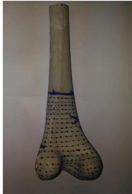
Fig. 4. Femur phantom model with markings for contact measurement
