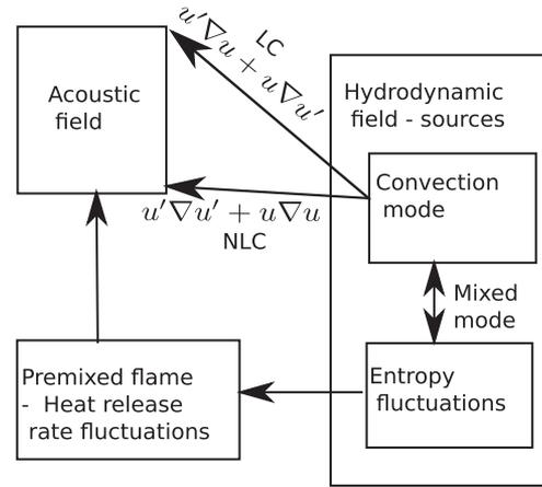
FIG. 1. Possible mechanisms that lead to the coupling of the flame with the acoustic, hydrodynamic, and entropy fields. Both the linear coupling (LC), discussed in this paper, and the non-linear coupling (NLC) are indicated. Heat release rate fluctuation serves as a source for the acoustic field. Hydrodynamic field causes both the convective mechanism and the entropy fluctuations, resulting from the non-uniform base flow, to couple and contribute to the acoustic field as a mixed mode.
