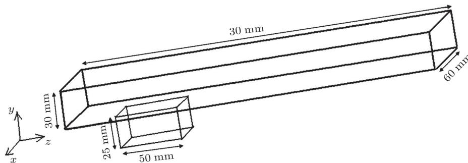
Fig. 2. Schematic diagram of three-dimensional cavity configuration.
