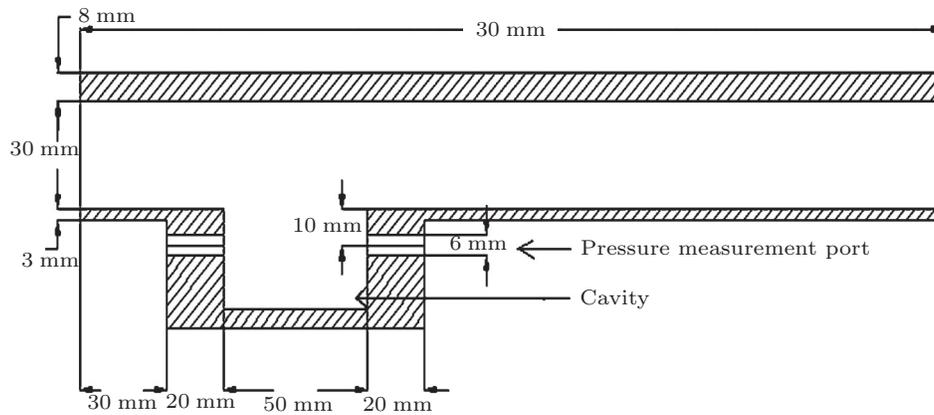
Fig. 1. Schematic of test section.
