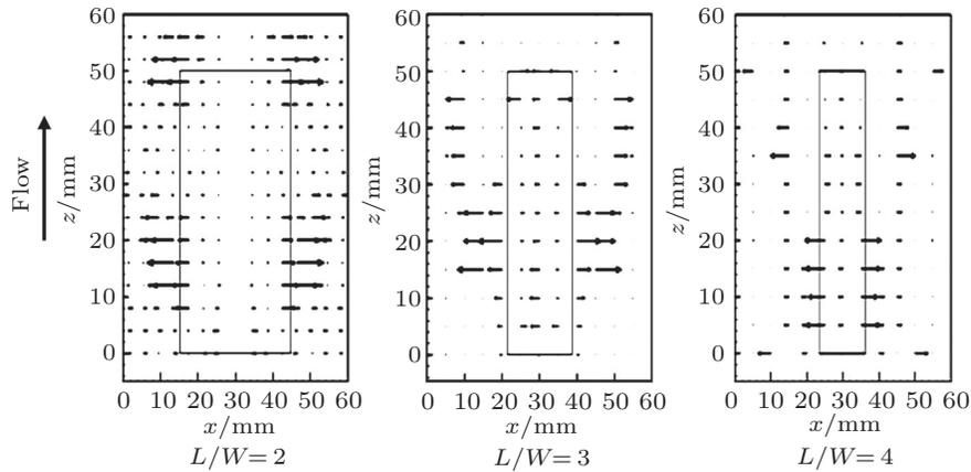
Fig. 3. Velocity vectors along a plane 2 mm above the cavity open top.
