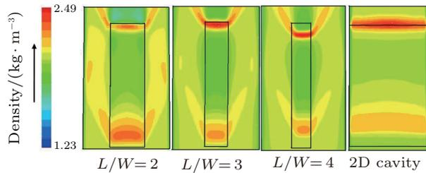
Fig. 9. Filled contours of density along a plane 2 mm above the test section floor.
