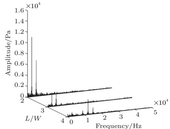
Fig. 5. Amplitude spectra of pressure oscillations (leading edge).
