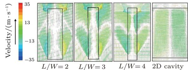
Fig. 8. Lateral velocity vectors in a plane 2 mm above the test section floor.
