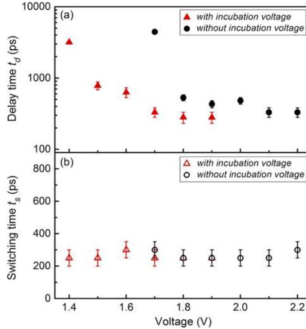
FIG. 3. (a) Dependence of delay time,  $t_d$ , and (b) switching time,  $t_s$ , on applied voltage pulse,  $V_A$  for both the cases of with ( $V_i$  of 0.3 V) and without incubation voltage ( $V_i$  of 0 V).
