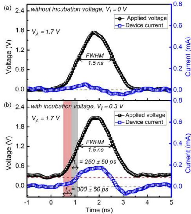
FIG. 4. Current-voltage characteristics of IST devices for the applied voltage pulse,  $V_A$  of 1.7 V with a full width half maxima (FWHM) pulse-width of 1.5 ns, rise time, and fall time of 1 ns (a) without incubation voltage, the device does not exhibit switching (b) with incubation voltage, reveals ultrafast *set* process of IST devices for the same  $V_A$  of 1.7 V within 1.5 ns.
