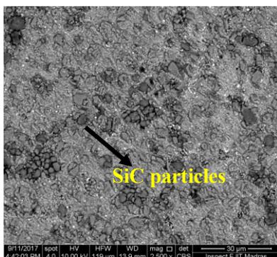
Fig. 1. Microstructure of Al-SiC MMC
