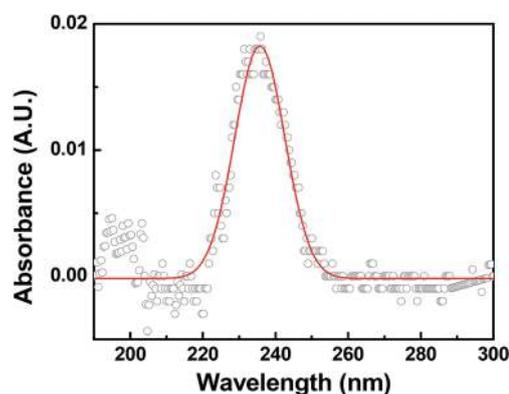
Fig. 8 Typical optical absorption spectra of cathode reservoir solution (recorded with Pt/MWNTs cathode in DF mode after 90 min reaction).
