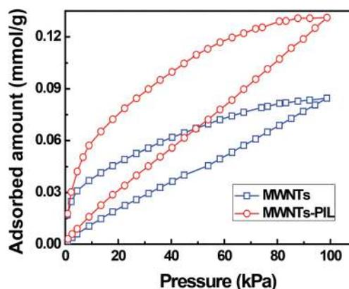
Fig. 4 Carbon dioxide adsorption properties of MWNTs and MWNTs–PIL at 283 K.
