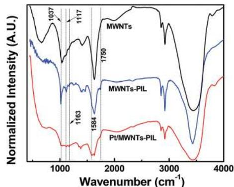
Fig. 3 FTIR spectrum of MWNTs, MWNTs–PIL and Pt/MWNTs–PIL.
