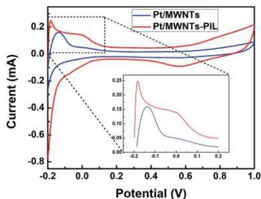
Fig. 5 Cyclic voltammogram of Pt/MWNTs and Pt/MWNTs-PIL electrode. Electrolyte: 1 M H<sub>2</sub>SO<sub>4</sub>, reference electrode: saturated Ag/AgCl electrode.
