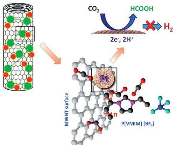
Fig. 12 Schematic representation of the mechanism behind the enhancement in performance.
