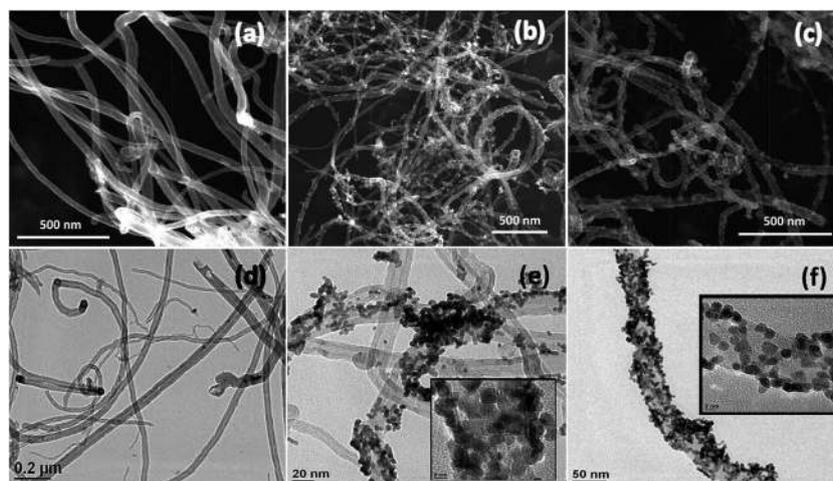
Fig. 1 FESEM images of (a) MWNTs, (b) Pt/MWNTs, (c) Pt/MWNTs–PIL and TEM images of (d) MWNTs, (e) Pt/MWNTs and (f) Pt/MWNTs–PIL (insets: respective high magnification images).
