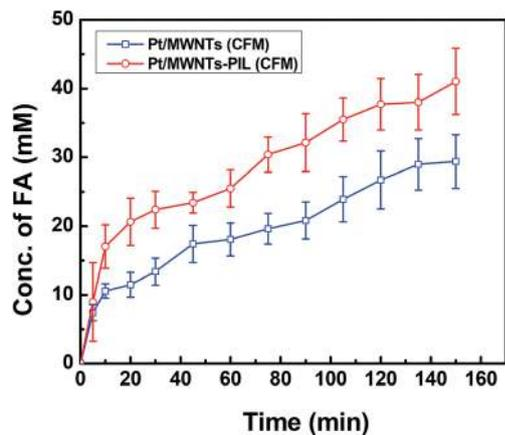
Fig. 11 Electrochemical formic acid (FA) formation from  $\text{CO}_2$  on Pt/MWNTs and Pt/MWNTs-PIL cathode PEM cell in continuous flow (CF) mode.
