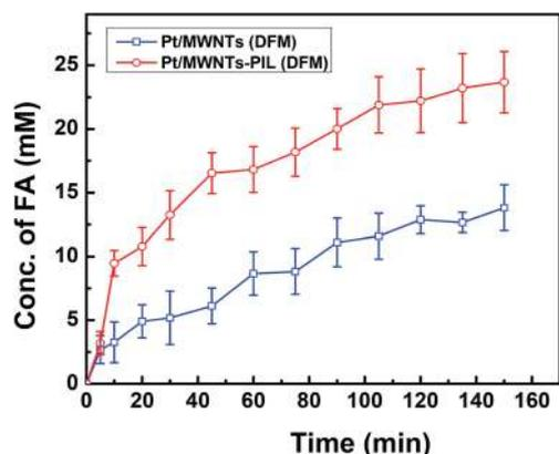
Fig. 10 Electrochemical formic acid (FA) formation from CO<sub>2</sub> on Pt/MWNTs and Pt/MWNTs-PIL cathode PEM cell in discontinuous flow (DF) mode.
