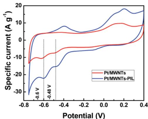
Fig. 6 Cyclic voltammogram of CO<sub>2</sub> reduction on Pt/MWNTs and Pt/MWNTs-PIL electrode. Electrolyte: CO<sub>2</sub> saturated 0.5 M KHCO<sub>3</sub>, reference electrode: saturated Ag/AgCl electrode.
