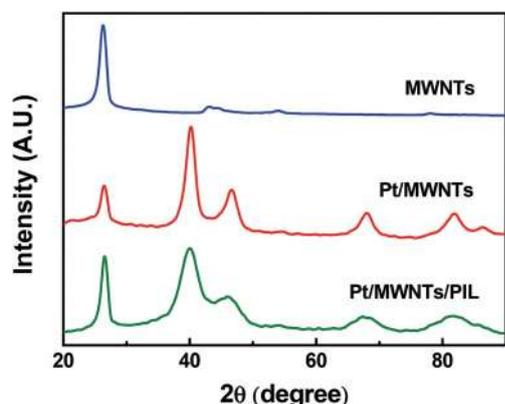
Fig. 2 X-ray diffractogram of MWNTs, Pt–MWNTs and Pt/MWNTs–PIL.
