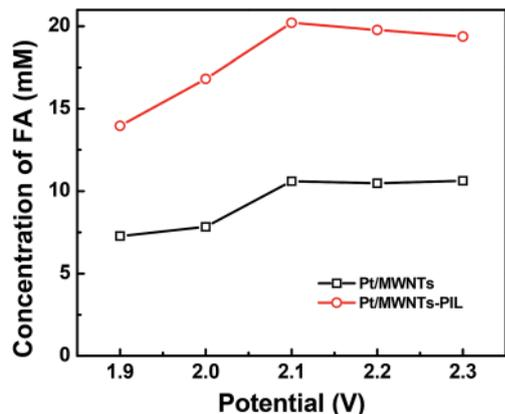
Fig. 9 Determination of working potential of PEM CO<sub>2</sub> conversion cell by discontinuous flow mode with 60 min conversion time per each data.
