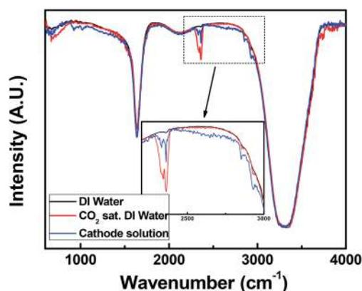
Fig. 7 FTIR spectrum of pure DI water, CO<sub>2</sub> saturated DI water and cathode reservoir solution (after 90 min of reaction).
