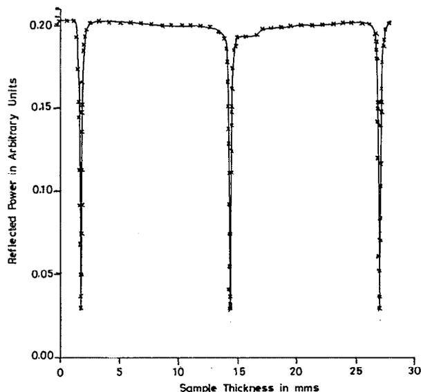
FIG. 2. The cavity resonances obtained for a lossy sample acetonitrile.
