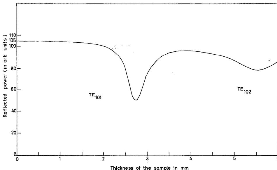
FIG. 1. The cavity resonances obtained for a nonlossy sample, benzene. The zero reading in  $x$  axis does not correspond to the actual zero thickness of the sample.
