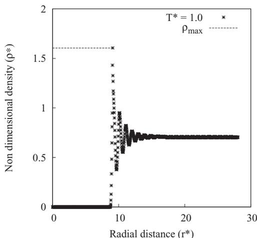
FIG. 13. Density profile of the Lennard-Jones fluid around nanoparticle at  $T^* = 1$  ( $\epsilon_r = 0.54$ ).
