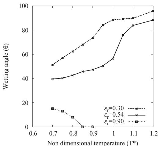
FIG. 7. Variation in wetting angle with temperature.
