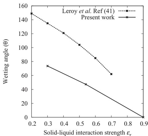
FIG. 8. Variation in wetting angle with interaction strength.
