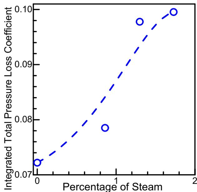
Fig. 15 Variation of total pressure loss coefficient with percentage of steam at  $M=0.52$
