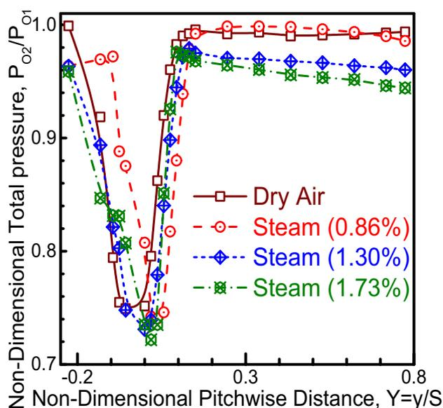
Fig. 13 Pitchwise distribution of non-dimensional total pressure at cascade exit at  $M=0.52$
