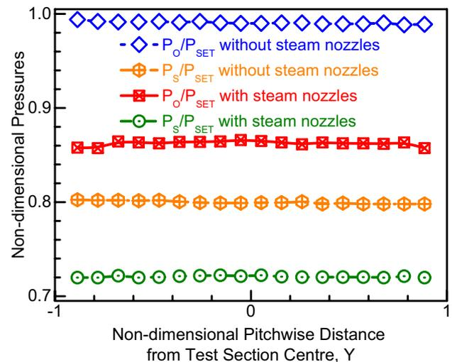
**Fig. 10** Cascade inlet flow traverses at  $M=0.52$
