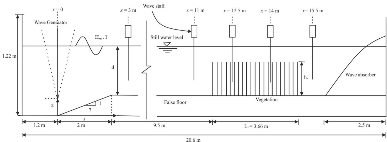
**Fig. 9** Definition sketch of the experiment setup
