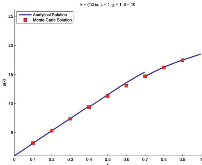
Figure 4. Analytical and Monte Carlo results for the solution of the Helmholtz equation plotted against length for  $k = \frac{\pi}{3}$ ,  $L = 1$ ,  $\chi = 1$ ,  $\delta = 10$ .
