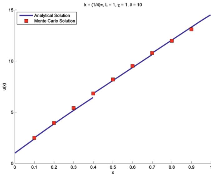
Figure 3. Analytical and Monte Carlo results for the solution of the Helmholtz equation plotted against length for  $k = \frac{\pi}{4}$ ,  $L = 1$ ,  $\chi = 1$ ,  $\delta = 10$ .
