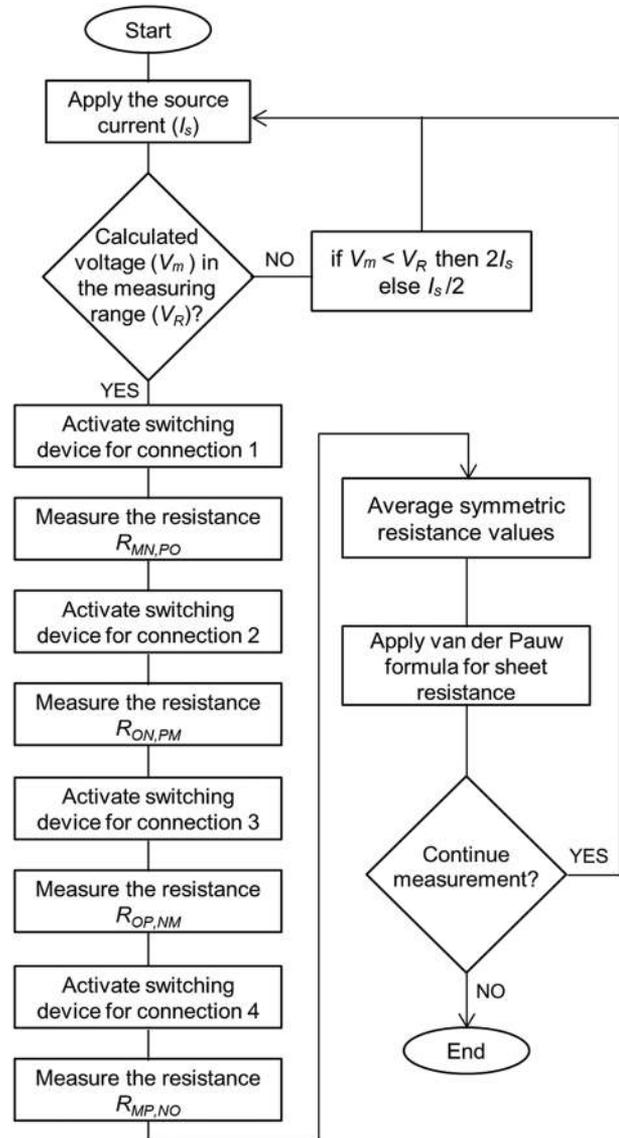
FIG. 4. Flowchart of the program to calculate the resistance as per the VDP method.
