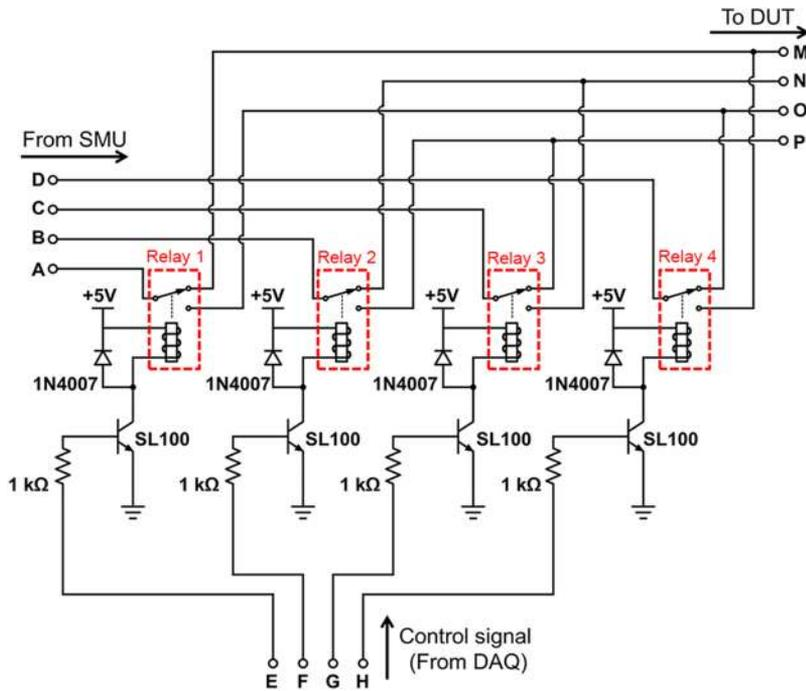
FIG. 2. Circuit diagram of the custom-built switching network board.
