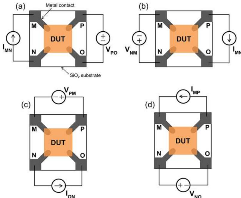
FIG. 3. Sample connections to identify the resistance according to the VDP method. Four connections from (a) to (d) with source and sense terminals have been mentioned to identify multiple resistance values.
