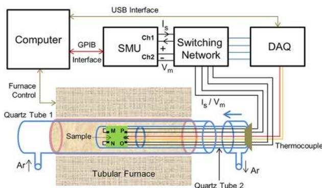
FIG. 1. Schematic of temperature dependent VDP resistance measurement setup. Tubular furnace is used to heat the sample, and a quartz based sample holder is designed for loading the sample at high temperature. Setup is fully automated and each instrument is controlled through LabVIEW.
