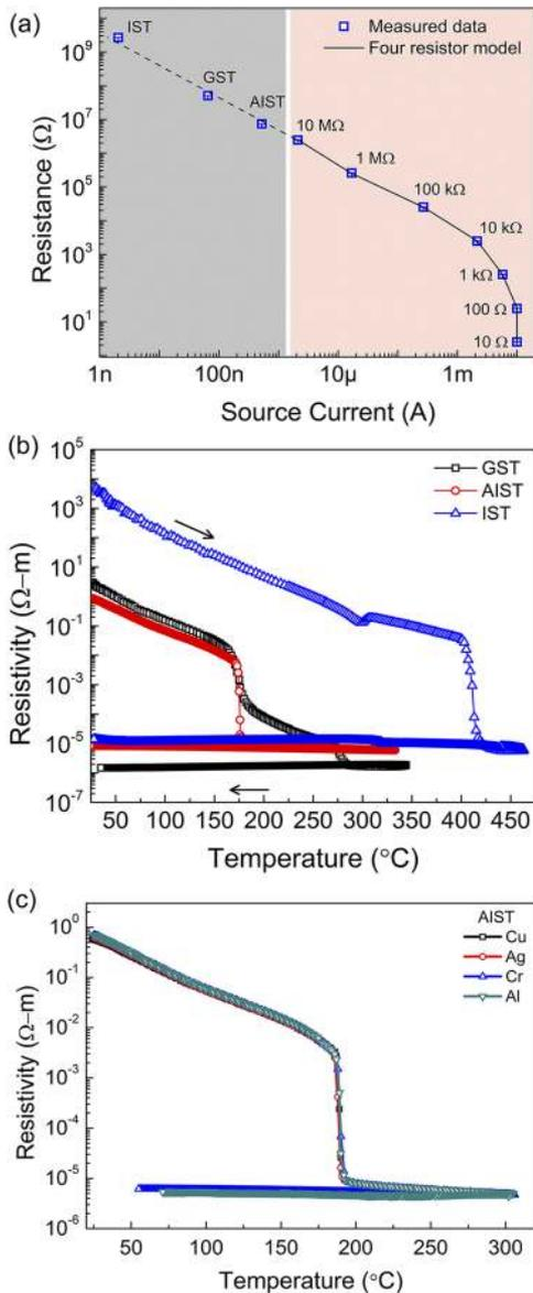
FIG. 5. (a) The calculated resistance values using the four-resistor model<sup>20</sup> and experimental data (symbol) and their fitting (line) for calibration of the setup. (b) Temperature dependent resistance of GST, AIST, and IST exhibits amorphous to crystalline phase transitions by means of rapid change in resistance during amorphous to crystalline phase transformation. (c) Resistivity measurement of AIST upon temperature using different metal contacts.
