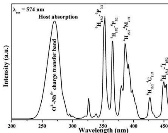
**Fig. 6** Excitation spectrum of  $\text{Ca}_{0.84}\text{Dy}_{0.08}\text{Na}_{0.08}\text{Nb}_2\text{O}_6$ .
