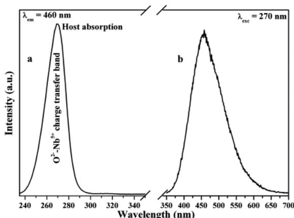
**Fig. 5** Excitation and emission spectra of  $\text{CaNb}_2\text{O}_6$ .
