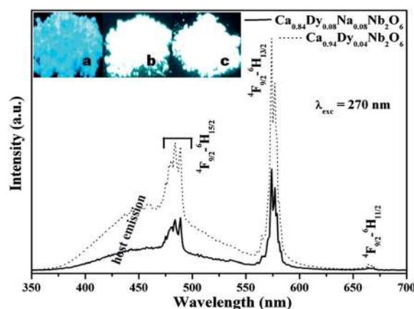
Fig. 10 Comparative emission spectra of  $\text{Ca}_{0.84}\text{Dy}_{0.08}\text{Na}_{0.08}\text{Nb}_2\text{O}_6$  and  $\text{Ca}_{0.94}\text{Dy}_{0.04}\text{Nb}_2\text{O}_6$  (inset shows the photoluminescence images of (a)  $\text{LaNbO}_4$  (b)  $\text{Ca}_{0.84}\text{Dy}_{0.08}\text{Na}_{0.08}\text{Nb}_2\text{O}_6$  and (c)  $\text{Ca}_{0.94}\text{Dy}_{0.04}\text{Nb}_2\text{O}_6$  irradiated with a 254 nm external lamp).
