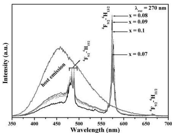
Fig. 7 Emission spectra of  $\text{Ca}_{1-2x}\text{Dy}_x\text{Na}_x\text{Nb}_2\text{O}_6$  ( $x = 0.07, 0.08, 0.09, 0.1$ ).
