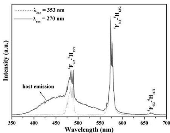
Fig. 8 Comparative emission spectra of  $\text{Ca}_{0.84}\text{Dy}_{0.08}\text{Na}_{0.08}\text{Nb}_2\text{O}_6$  under host and 353 nm excitations.
