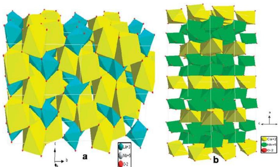
**Fig. 11** Crystal structures of  $\text{LaNbO}_4$  ( $\text{NbO}_6$  octahedra are represented in blue and  $\text{LaO}_8$  ions with yellow) and  $\text{CaNb}_2\text{O}_6$  ( $\text{NbO}_6$  octahedra are represented in green and  $\text{CaO}_6$  ions with yellow).
