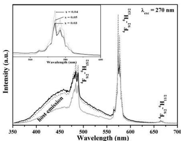
Fig. 9 Emission spectra of  $\text{Ca}_{1-x}\text{Dy}_x\text{Nb}_2\text{O}_6$  ( $x = 0.03, 0.04, 0.05$ ).
