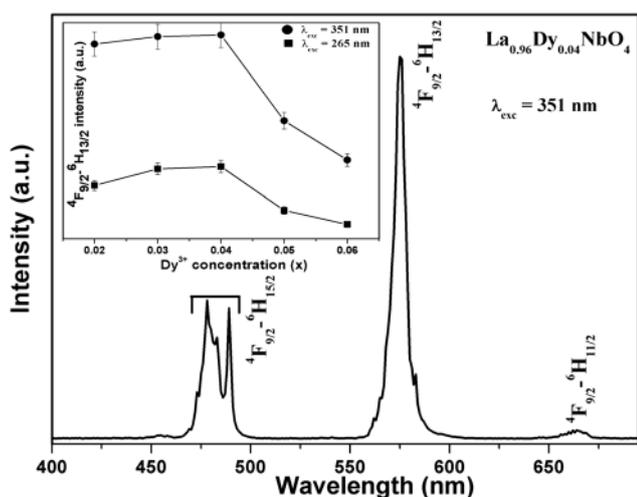
**Fig. 4** Emission spectrum of  $\text{La}_{0.96}\text{Dy}_{0.04}\text{NbO}_4$  under 351 nm excitation (inset shows concentration dependence of  $\text{Dy}^{3+}$  emission intensity in  $\text{La}_{1-x}\text{Dy}_x\text{NbO}_4$  under both host and 351 nm excitations).
