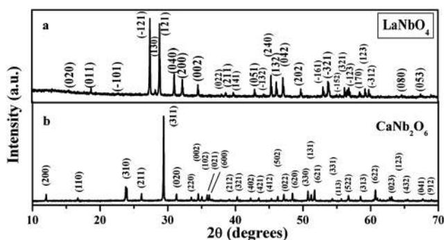
Fig. 1 X-Ray powder diffraction patterns of  $\text{LaNbO}_4$  and  $\text{CaNb}_2\text{O}_6$ .
