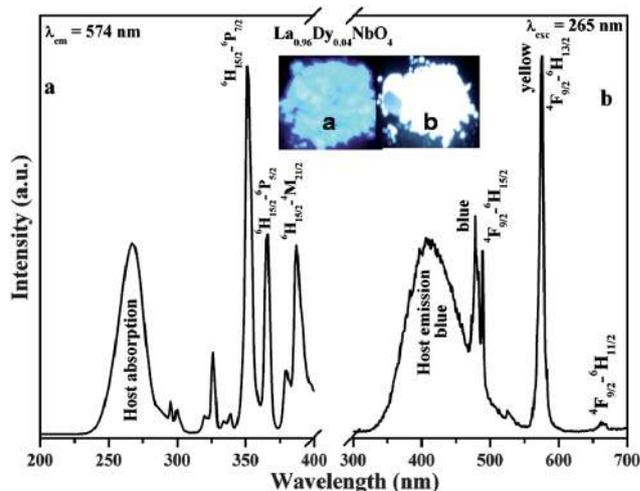
Fig. 3 Excitation and emission spectra of  $\text{La}_{0.96}\text{Dy}_{0.04}\text{NbO}_4$  (Inset shows images of (a) undoped; (b) 0.04  $\text{Dy}^{3+}$  doped  $\text{LaNbO}_4$  under 254 nm external lamp).
