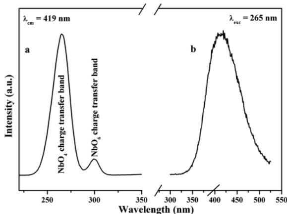
Fig. 2 Excitation and emission spectra of  $\text{LaNbO}_4$ .
